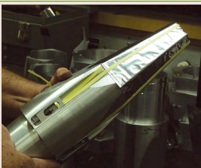
A completed detector element consisting of a BaF 2 crystal wrapped with black plastic to keep out external light, a 3-in. photomultiplier tube, and an aluminum enclosure.
