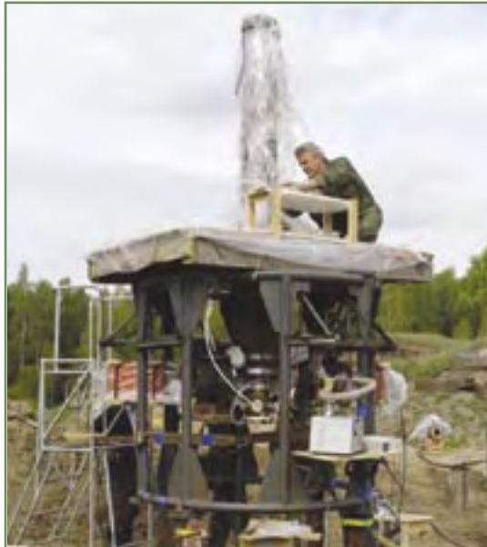
Russian High-Explosive Pulsed-Power System. The system delivers electrical energy comparable to Atlas but is single use.
