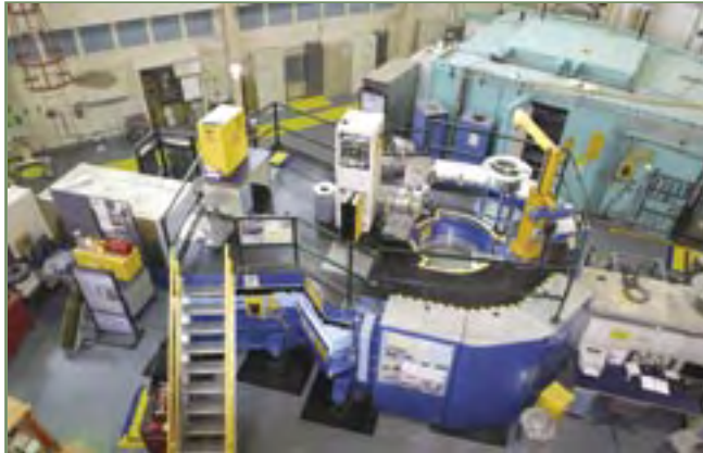
The NPDF is located at flight path 1 at the Lujan Neutron Scattering Center. The instrument was recently upgraded for a total cost of $1.1M shared by the National Science Foundation, several academic institutions, and LANL. The NPDF is now among the world's leading diffractometers, specialized in the study of the atomic structure of complex materials.
