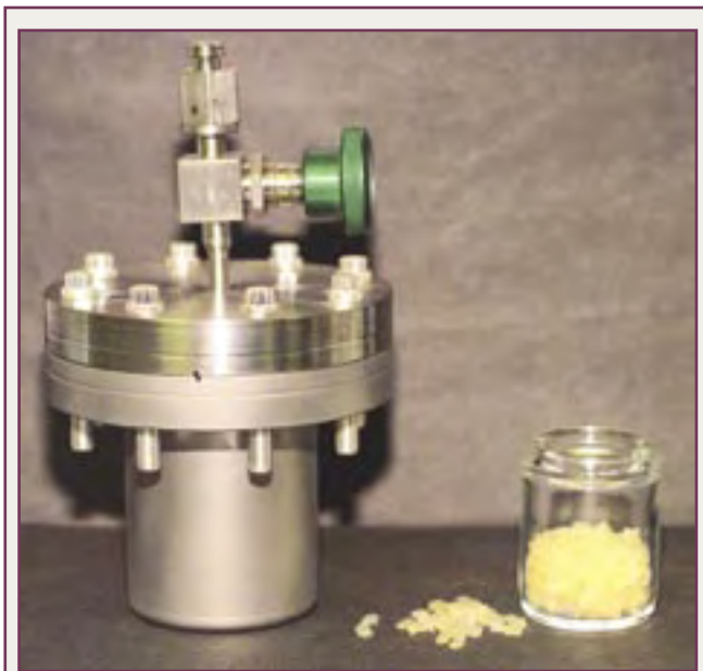
Container used in the CAS and jar with Estane pellets. Over 1,000 of these containers containing samples, made up of 25 different combinations of constituents of PBX 9501, were placed in ovens and held at a fixed temperature for specified intervals of time. Decomposition gases were extracted from each container and the chemical makeup determined.
