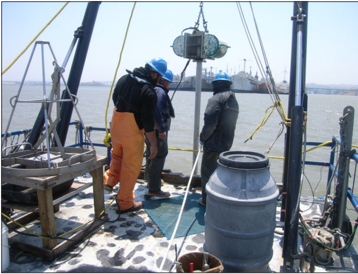
Photo, above: Scientist deploying Vibracore for sampling.
