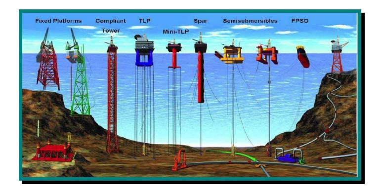
columns that are partially submerged. Semisubmersibles can operate in a wide range of water depths, including deep water. They are usually anchored with eight to sixteen anchor chains, which are computer controlled to maintain position. Semisubmersibles can be used for most aspects of offshore drilling. The size of a semisubmersible can be vast, comparable to a floating skyscraper.
