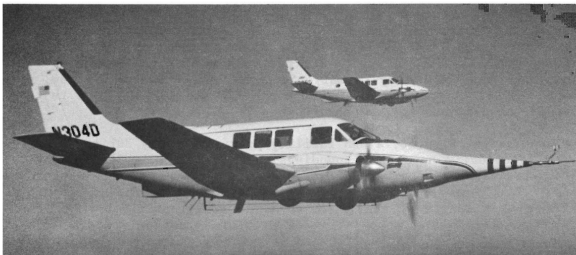
Figure 2.4. The research aircraft operated by the National Center for Atmospheric Research. The Queen Air is instrumented for low level turbulence measurements.
