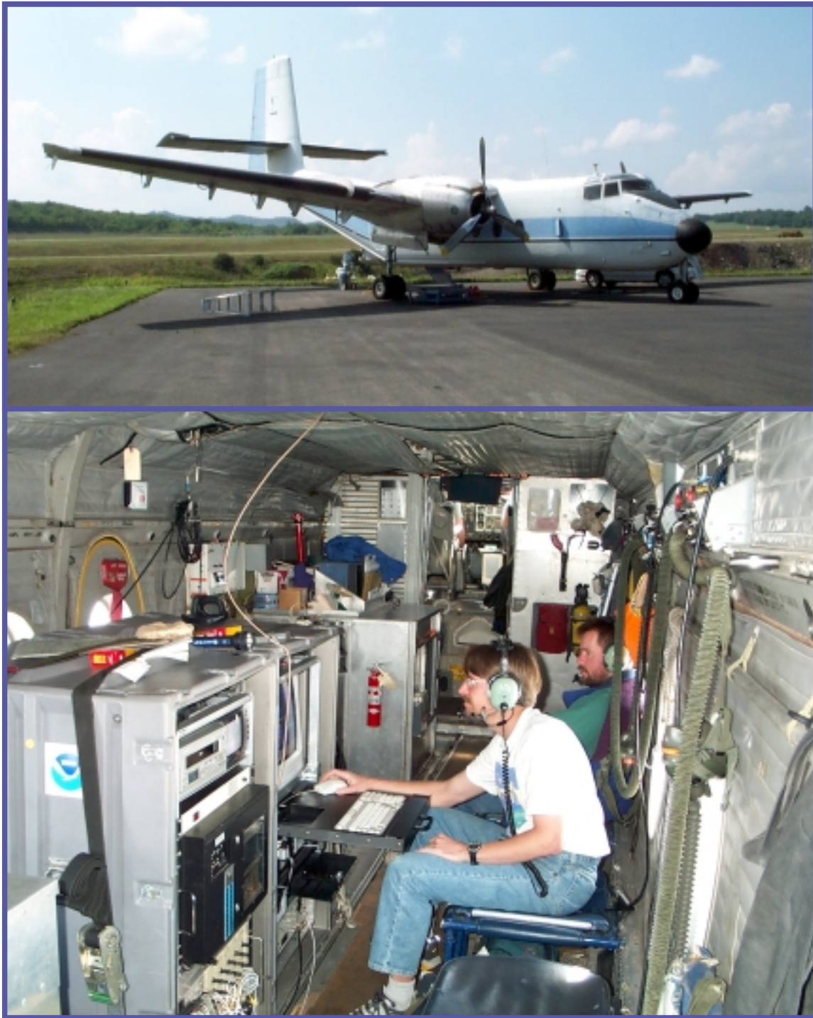
The NOAA ozone/aerosol lidar was carried aboard a deHavilland Caribou aircraft (top), during the 1999 SOS Nashville field campaign. This aircraft is specially configured for remote sensing studies with a crew of two or three scientists to operate the lidar, evaluate the measurements, and direct the mission (bottom). The airborne lidar provided three dimensional measurements of ozone and fine particle concentrations over the Nashville area (see pages 16-18), enabling researchers to track the evolution and transport of these pollutants throughout the region.
