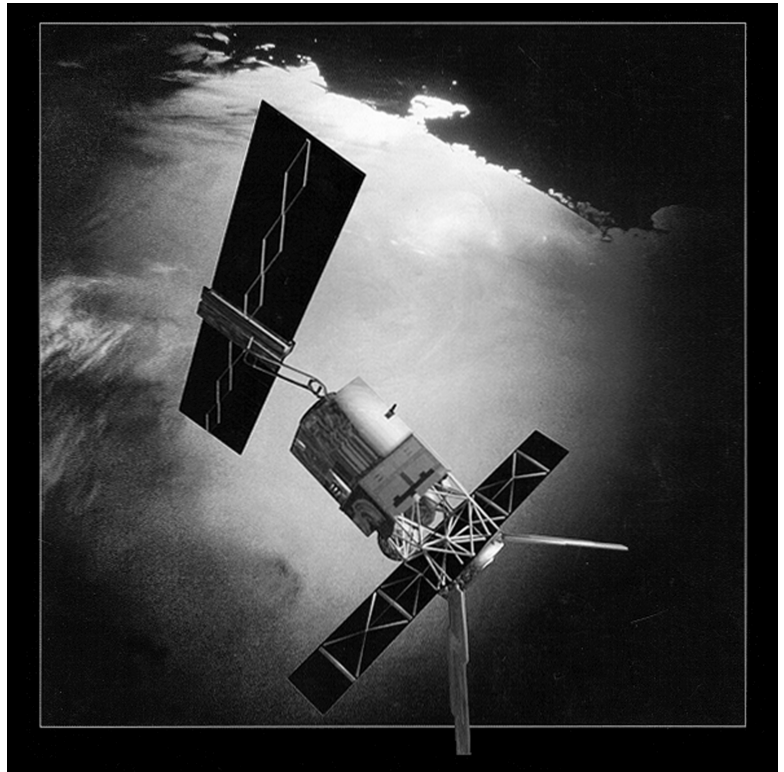
▲ Figure 1. Artist's rendition of the European Space Agency's ERS-1 satellite, which operated from 1991 to 1996. Data collected via the satellite was used to extend existing altimetric gravity fields of the global ocean (Laxon and McAdoo, 1994, Sandwell and Smith, 1997). Figure reproduced from The Data Book of ERS-1: The European Remote Sensing Satellite , European Space Agency, esa BR-75, April 1991.
