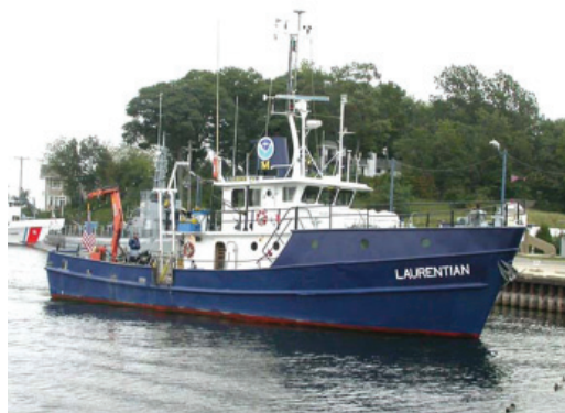
▲ R/V Laurentian was one of the first NOAA research vessels converted to operate on bio-based fuel and lubricants.
