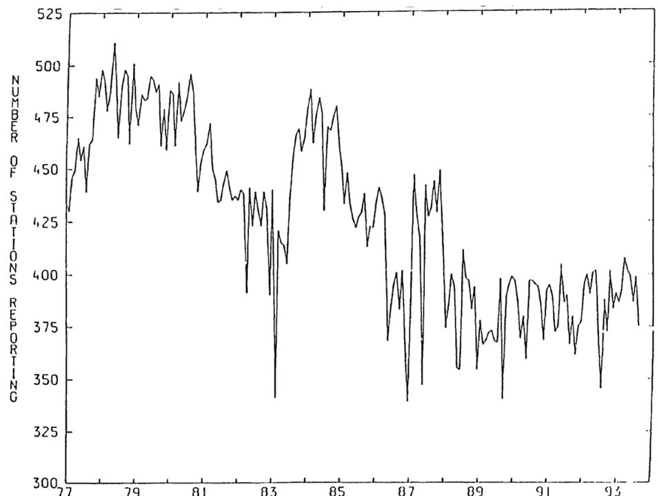
▲ Figure 5. Number of monthly "CLIMAT TEMP" messages (containing monthly upper air temperature summaries) by year received at the UK Meteorological Office through the Global Telecommunications System.
