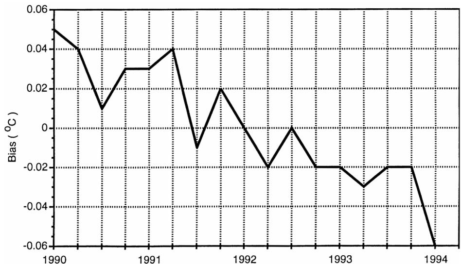
▲ Figure 3. MSU2R tropospheric temperature bias (plotted by year) attributed to diurnal sampling changes due to orbital satellite drift (Christy, *et al.*, 1995)
