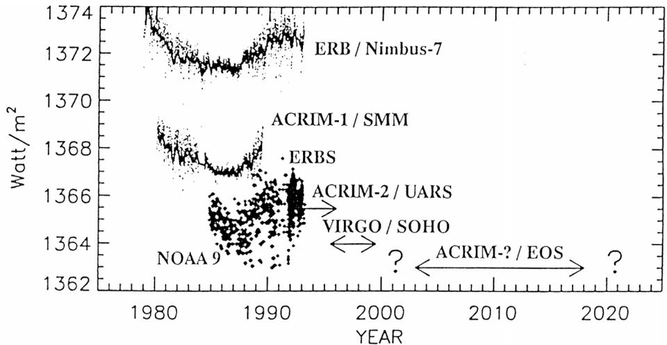
▲ Figure 4. Changes in total solar irradiance as measured from different satellites and instruments (adapted from NRC, 1994).
