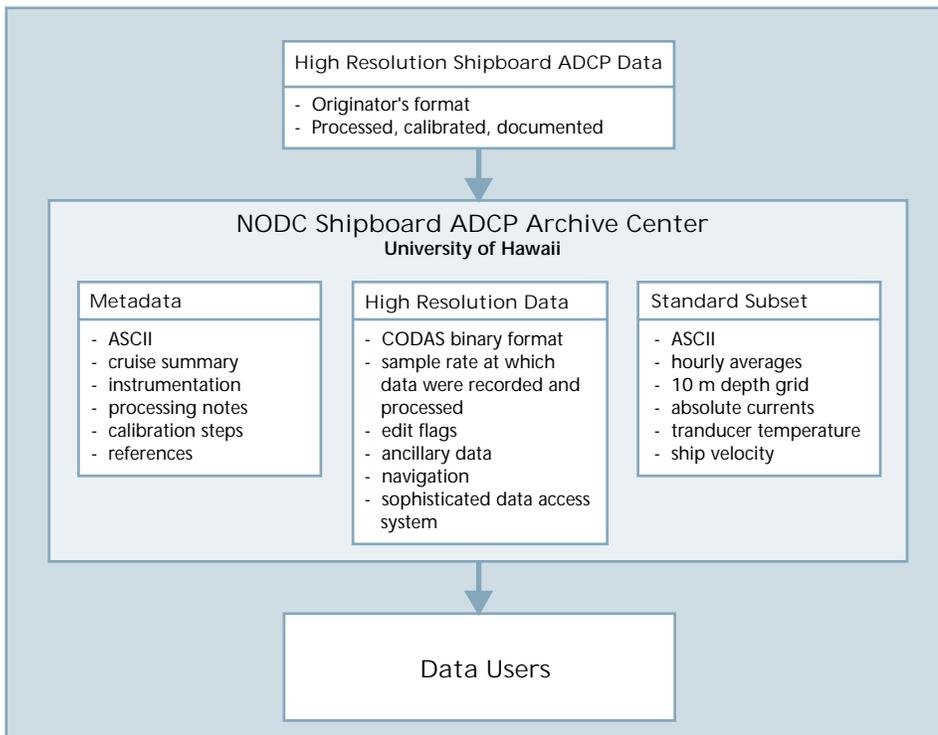
▲ **Figure 2.** Flow diagram of data processing, archival, and distribution procedures for shipboard ADCP data sets received at the Shipboard ADCP Center (SAC).
