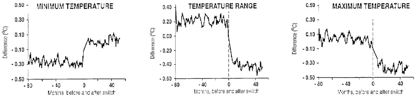
▲ Figure 1. Average differences of temperature between stations prior and subsequent to the switch from liquid-in-glass maximum-minimum thermometers in a wooden Cotton Region Shelter to a thermistor in a plastic "Beehive" shelter (from Quayle *et al.*, 1991).
