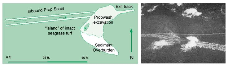
Finally, the propwash excavation by the boat engines caused sediment to become deposited behind the boat on top of unimpacted seagrass (above left). Blow-out scars, entrance and exit tracks, and sediment deposits are all visible in the aerial photograph (above right).
