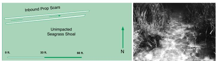
The diagrams on this page were created to document the sequence of events that occurred when a twin-engine boat grounded on a seagrass flat within the Sanctuary. First, the boat propellers dredged parallel prop scars across the seagrass flat (above left). The severity of a scar left by a propeller is apparent in the underwater photograph (above right).
