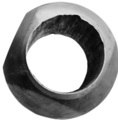
Figure 10: DSSV Ball cut by wireline (slickline) work done through the valve.
