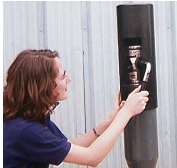
Figure 3: Photograph of a safety valve which has been cutaway and made-up on top of a section of drillpipe.
