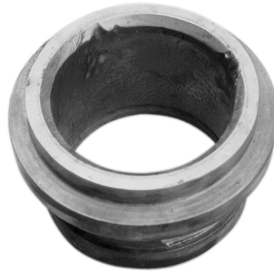
Figure 9: Erosion of Seat by Drilling Fluid in over-closed valve.
