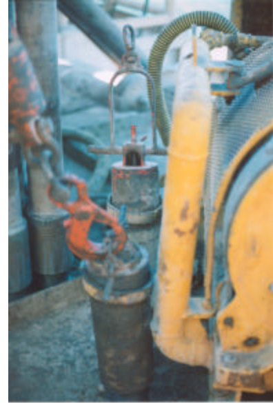
Figure 44: DSSV and Inside BOP on Rig Floor Ready to Stab on Drillstring if Needed
