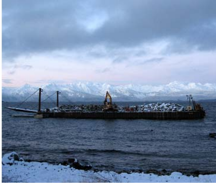
Figure 1: Barge carrying quarry rock anchored at Yankee Cove with the Chilkat mountains behind. Photo Credit: Allan Culbreath.
