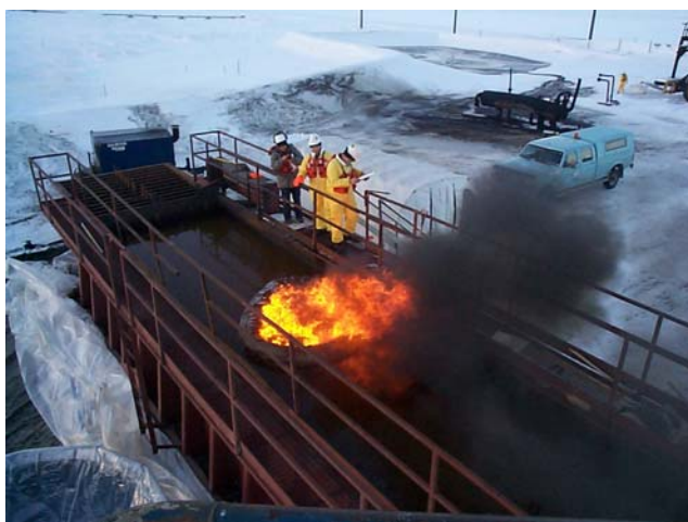
Figure 7: Test burn on frazil, or slush, ice.
