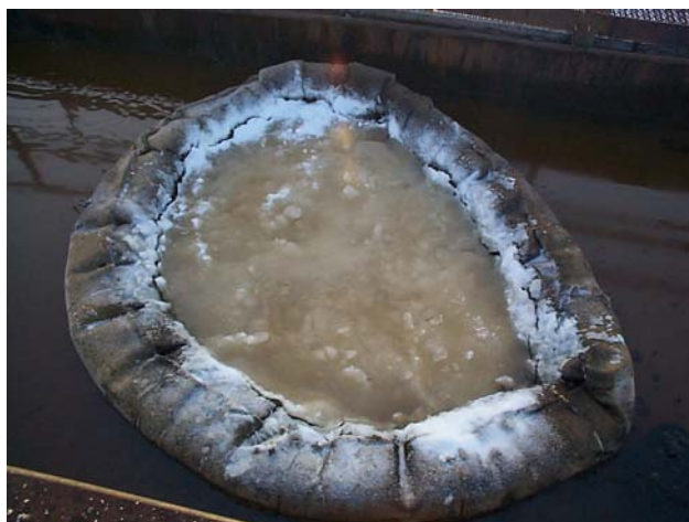
Figure 6: Fresh frazil, or slush, ice in ring prior to adding oil.
