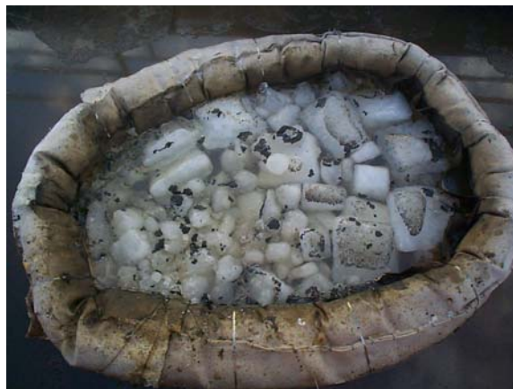
Figure 5: Brash ice after burn and residue recovery.
