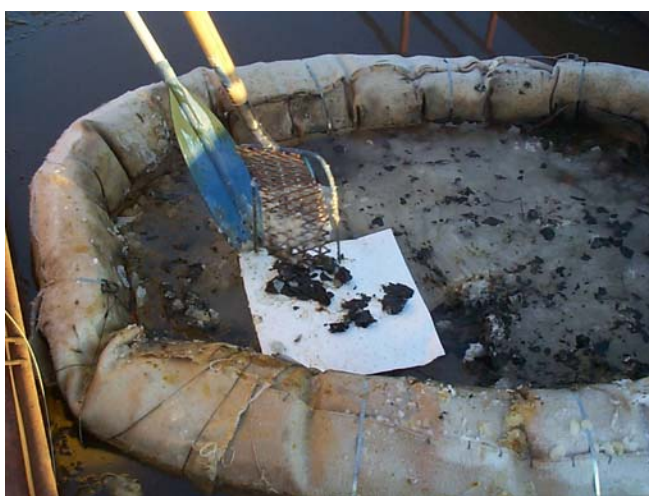
Figure 8: Recovering residue from burn ring after burn on frazil, or slush, ice.
