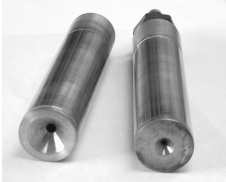
Figure II.1.7 Photograph of the 5 mm and 2 mm sharp edged orifice nozzles. The 1 mm diameter orifice nozzle has identical dimensions.
