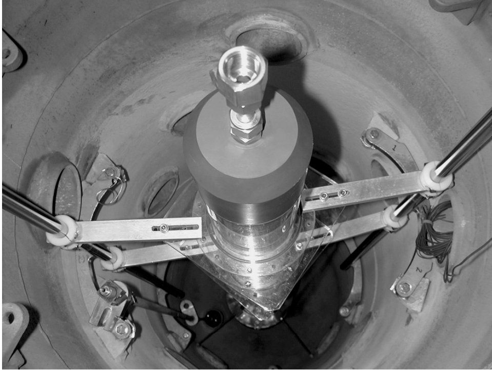
Figure II.1.15 Photograph of the water tunnel mounted inside the pressure vessel.
