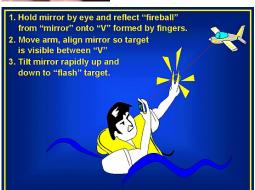
miles and generally the flash will be visible up to 50 miles, depending upon atmospheric conditions. The record rescue from one is 105 miles at sea. Direct up to 6 million candlepower of reflected sunlight onto the rescue target with pinpoint accuracy. A mirror will even work on bright overcast days and with moonlight, though with much reduced range. (Signal mirror will be inside the flotation vest stowage pocket.)
