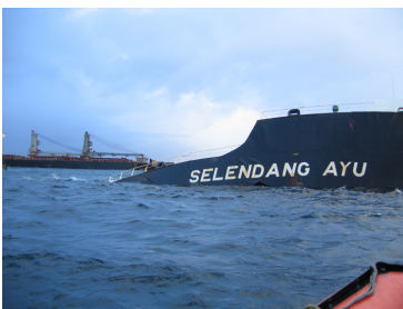
Broken sections of the Selendang Ayu before sinking. The bow section is in the foreground; the stern section in the background.
