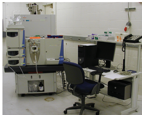
LC-ICR-LTQ mass spectrometer for high resolution mass measurement
