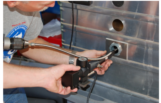
LANL personnel use an endoscopic tool mounted on a fiberscope to render safe a mock explosive device through a small breach in the device casing.
