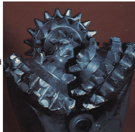
The teeth of the roller-cone drilling bit are equipped with abrasive inserts made of our diamond nanocomposites, which stand up to the intense friction, impact, and heat of down-hole drilling environments in the oil and natural-gas industry.
