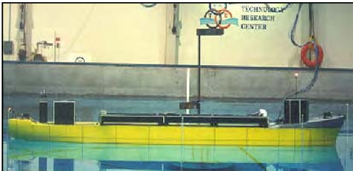
Figure 7: FPSO Model in Wave Basin
