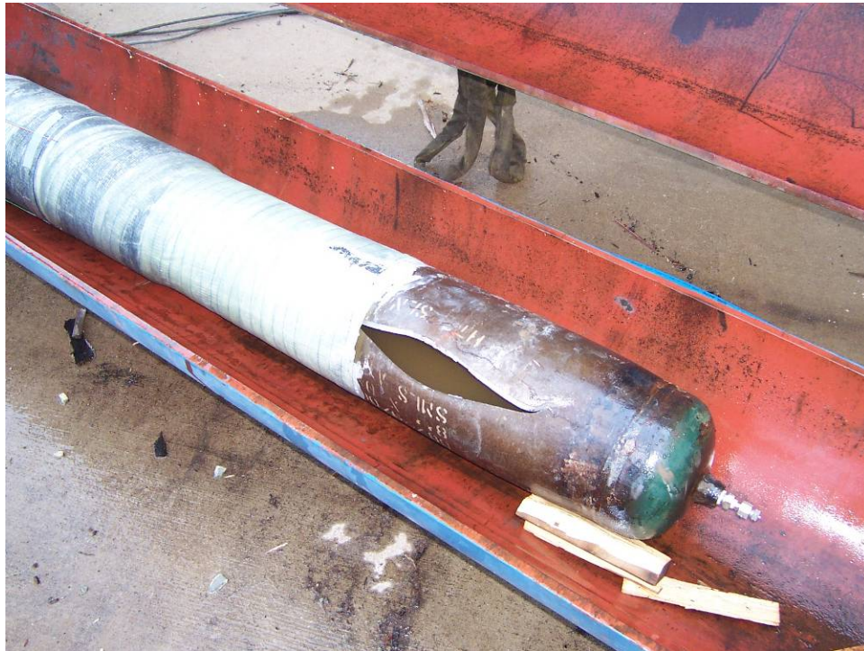
Figure 8 – Failure in burst sample using Product C
