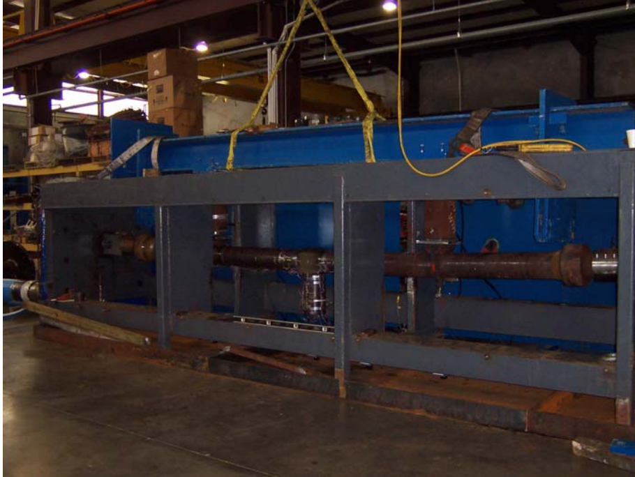
Figure 6 – Load frame used for pressure-tension-bend testing
