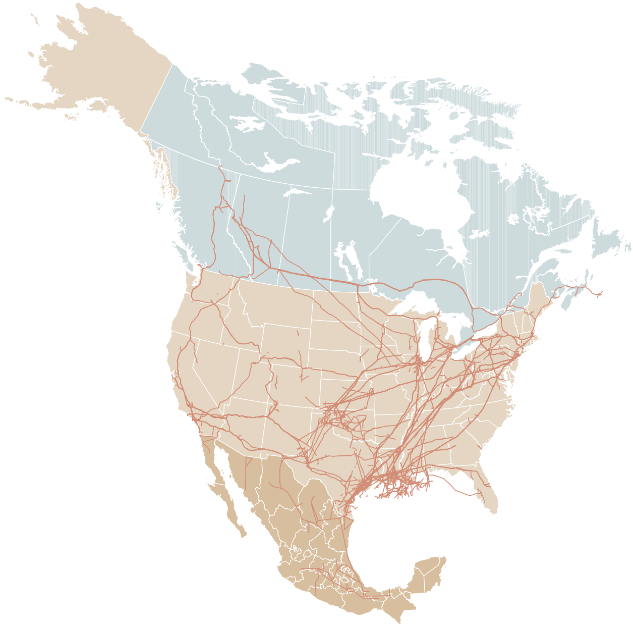
FIGURE 43 NORTH AMERICAN PIPELINE GRID (24" DIAMETER AND GREATER)
