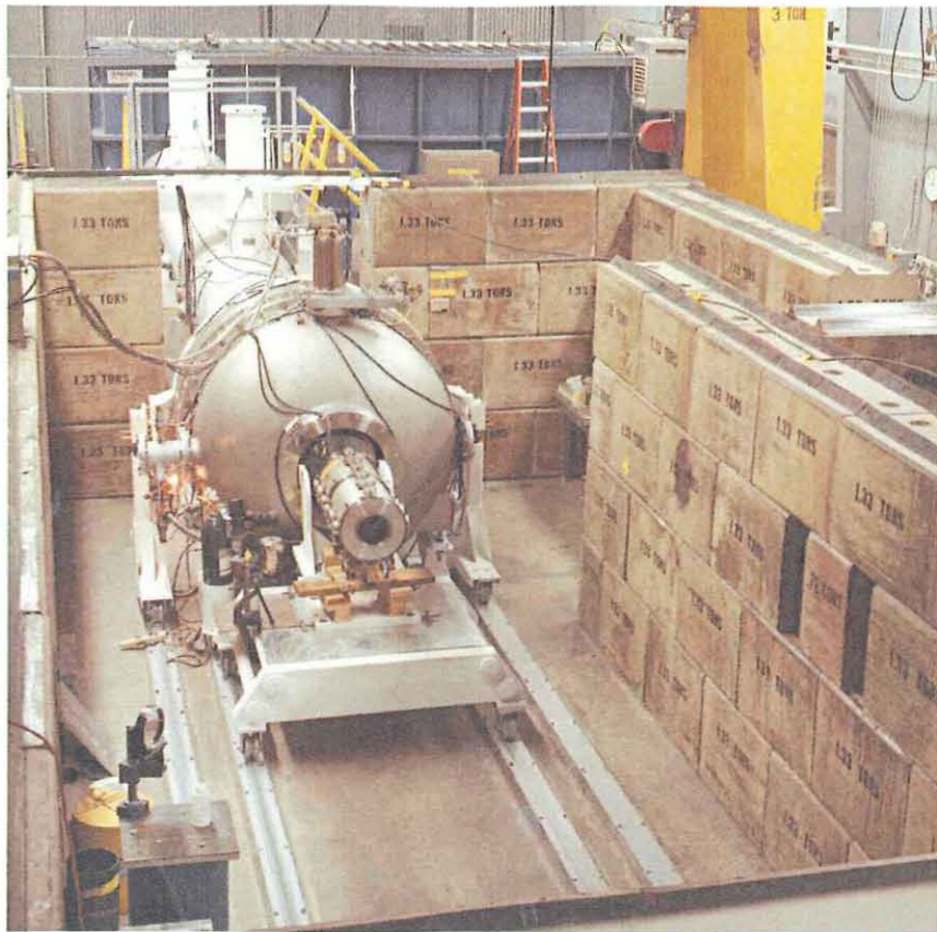
REX in 1988 surrounded by magnetite-loaded concrete shielding blocks (TA-15-203), photo courtesy of Rae Ridlon
