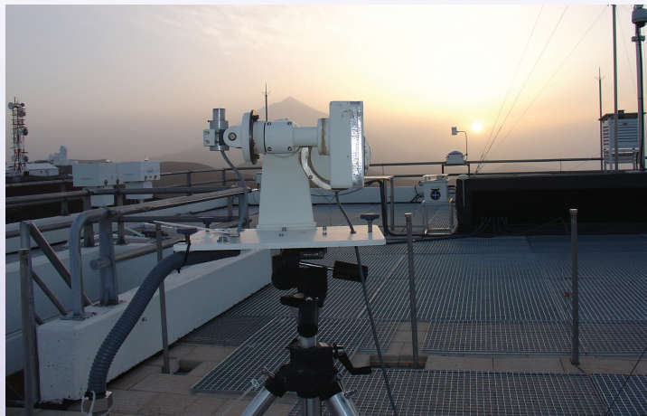
Photo 3. Izaña Observatory terrace during a moderate Saharan event. The tripod in the foreground holds the UV-spectrometer optics and stepper motor for off-axis measurements. In the back the housing of the scanning spectrometer located outdoor.
