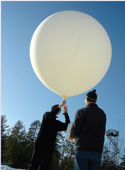
Launching ozonesondes from Sodankylä during SAUNA using a rubber balloon.
