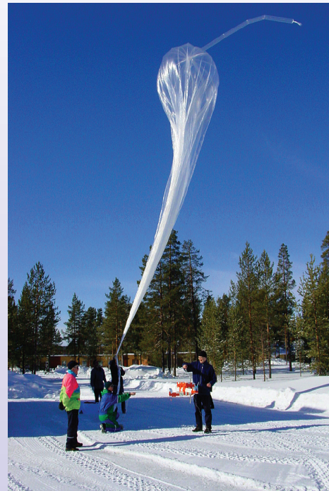
Launching ozonesondes from Sodankylä during SAUNA using a polyethylene balloon.
