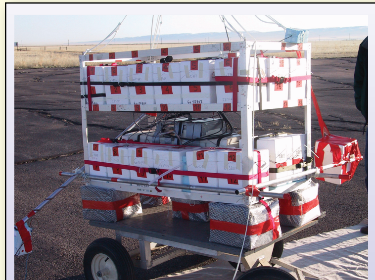
Sondes on the gondola ready for launch during the BESOS campaign.
