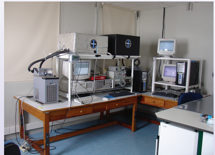
Photo 4. INTA PDA UV/Vis spectrometers are hosted in a laboratory located on the top floor of Izaña tower. Sunlight from the optical devices located on the terrace reach the instruments by means of a quartz fiber-bundle. Spectrometers are thermally regulated to minimize spectral shift and stretch.
