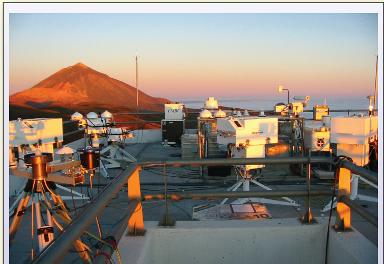
Photo 1. The double monochromator Brewer Spectrophotometer triad over the observation tower roof at the Izaña Observatory with other instruments.
