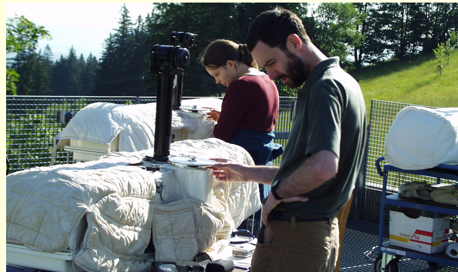
Final calibration after the refurbishment of the two Halley Bay Dobson instruments. Photo: Ulf Köhler.
