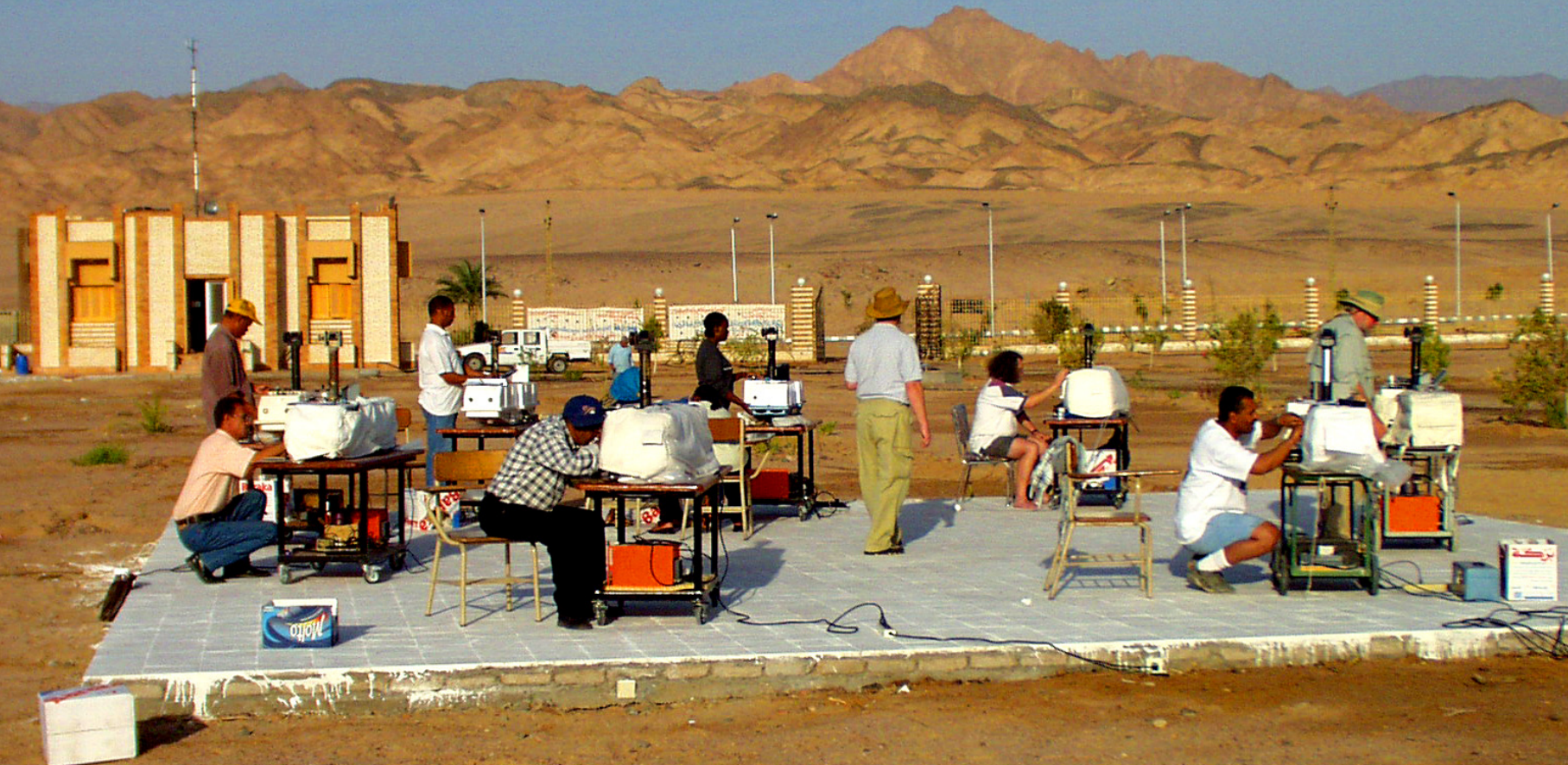
Intercomparison of Dobson spectrophotometers at Dahab, Egypt in February/March 2004. Photo: Ulf Köhler.
