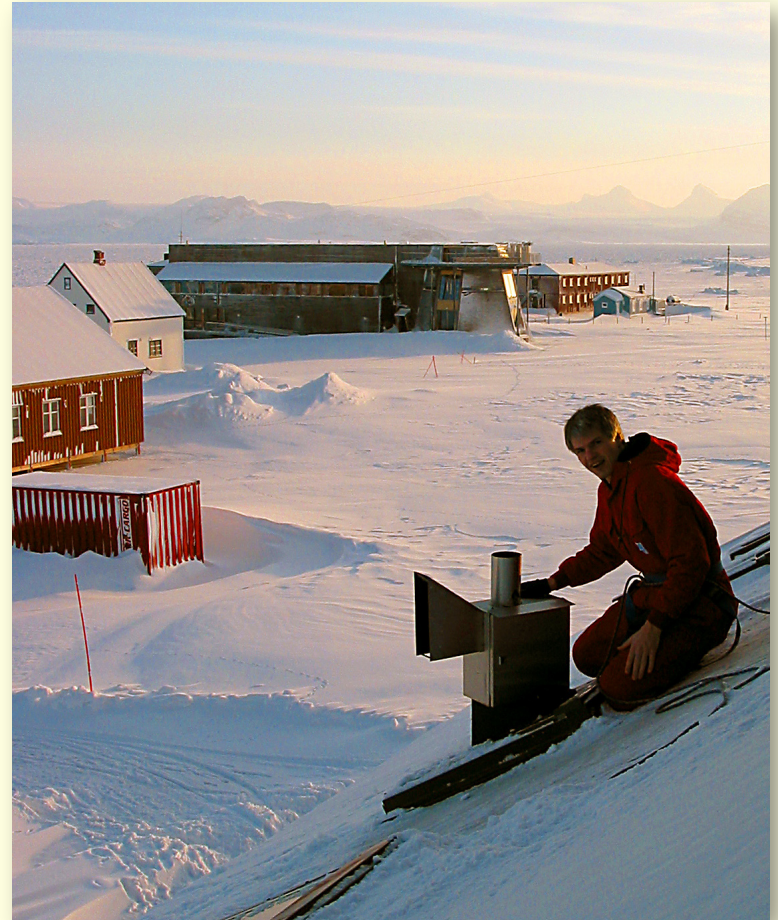
Folkard Wittrock adjusting the optical head of the MAX-DOAS instrument on the roof of the NDSC building at Ny-Ålesund. Photo: Hilke Oetjen, courtesy of IFE, University of Bremen
