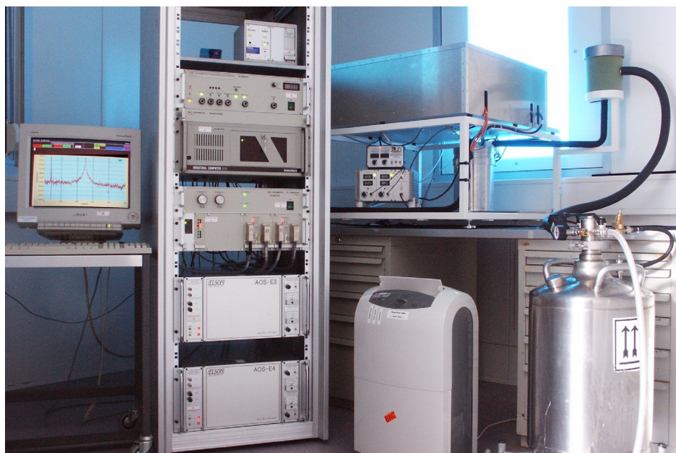
Figure 1. View of the microwave radiometer SOMORA located at the aerological station of Payerne.
