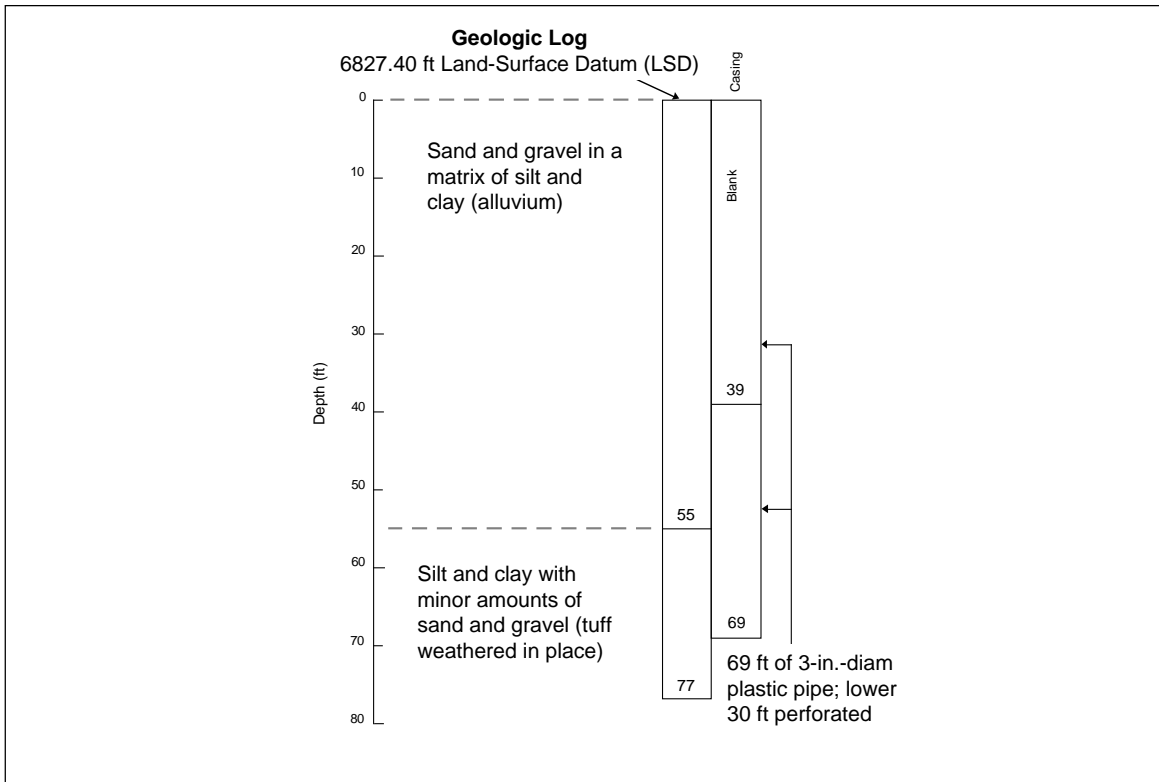
Fig. VI-K. Mortandad Canyon observation well MCO-7, completed October 1960, water level 39.7 ft (Baltz et al. 1963).
