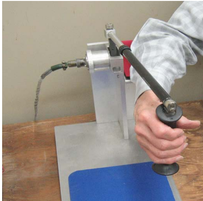
Fig. 4a. The Fine Motor Control Apparatus. Picture shows the handgrip and the position of the subject's arm during testing.
