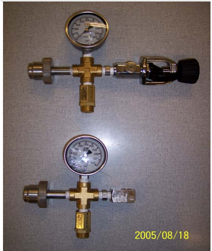
Photo of SCBA adapters now available to the NOAA Fleet. Top is SCUBA-to-SCBA, bottom is Compressor-to-SCBA adapter.
