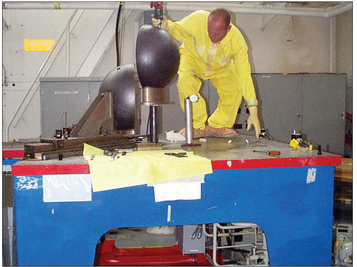
Jim Dyson of Advanced Nuclear Technology guides hoisting of the uranium reflector from the Flat Top criticality machine in preparation for the machine's move from Technical Area 18, its home since 1958, to TA-35. Los Alamos National Laboratory photo
