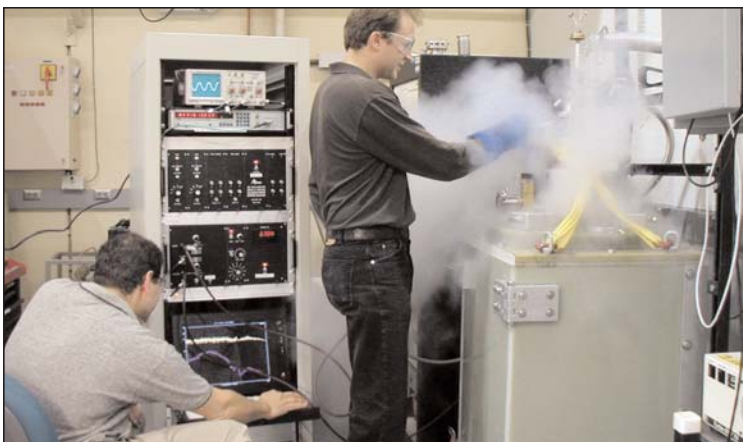
Chuck Mielke (seated) and Neil Harrison of the National High Magnetic Field Laboratory (NHMFL) prepare an experiment with a 60T short pulse magnet. The clouds are from the liquid nitrogen used to cool down the cryostat that holds the experiment inside the magnet. Mielke works with the data acquisition computer. Photo courtesy of NHMFL
