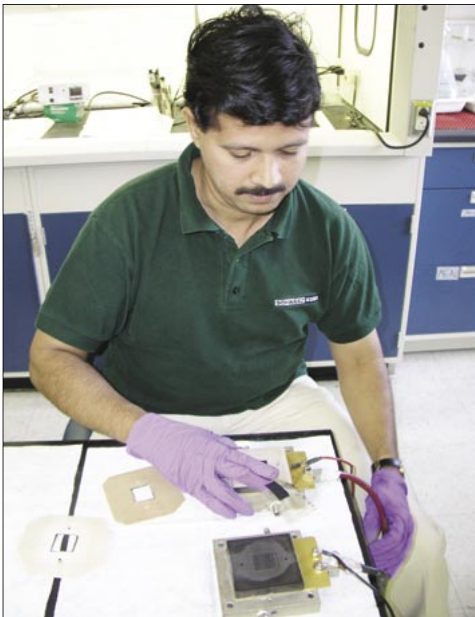
Rajesh Bashyam of Sensors and Electrochemical Devices assembles a polymer electrolyte fuel cell for testing in one of the Laboratory's fuel-cell laboratories. Photo by Karen Kippen of Communication, Arts, and Services
