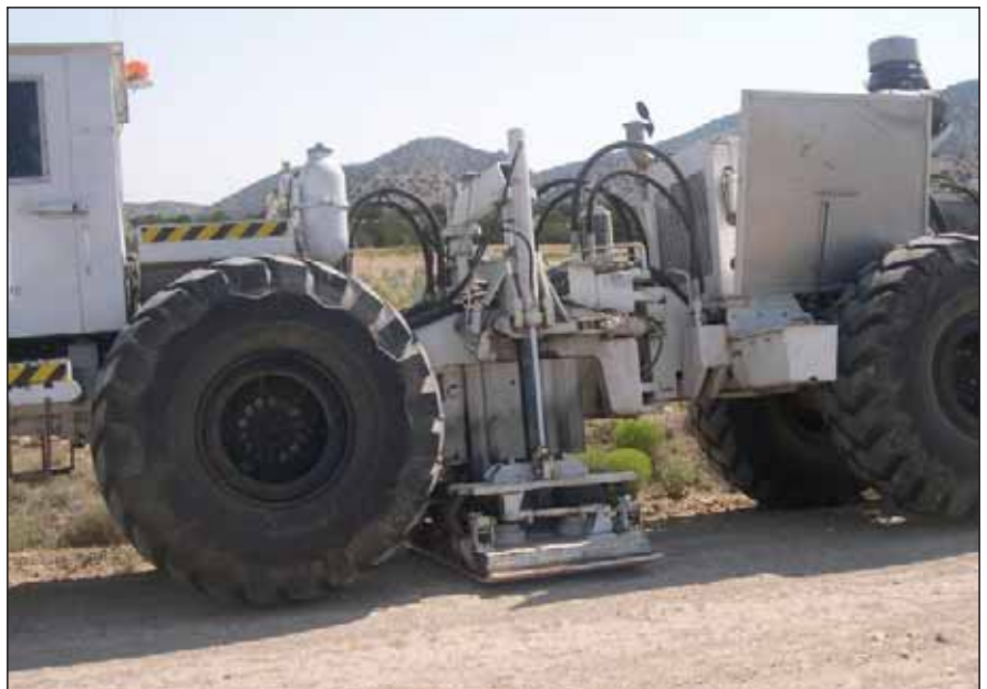
Above is a vibroseis truck, which is used as the source of seismic waves to image underground structure. The truck was provided to this year's SAGE program by Input/Output Inc.
