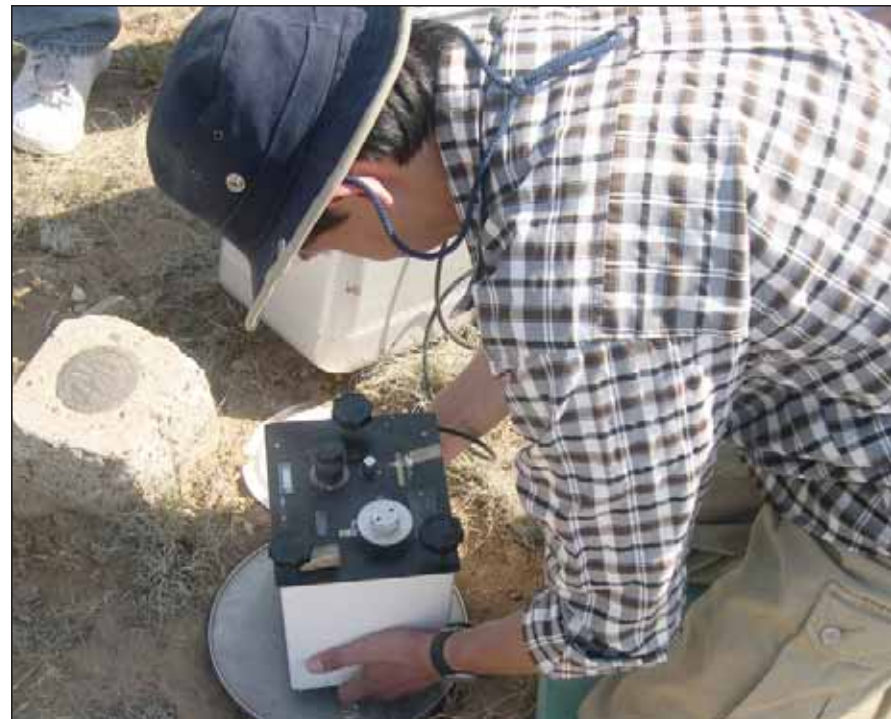
A student in the Laboratory's Summer of Applied Geophysical Experience (SAGE) program measures Earth's gravity field using a gravity meter.
