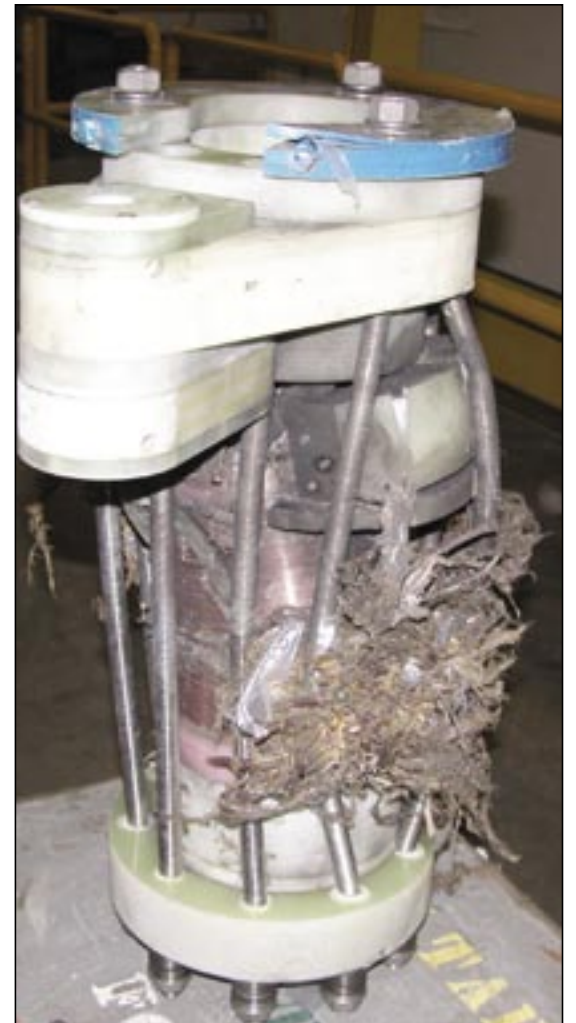
Left: A view of the 80-tesla magnet on the bench during final assembly prior to testing. The magnet windings are in the central region. Two nested solenoid coils comprise the 80-tesla. The inner solenoids construction is nearly identical to the insert magnets used for the 100 Tesla Multi-Shot Magnet program. Right: A view of the inner "insert" coil of the 80-tesla magnet. The magnet assembly is intact. Ironically the most highly stressed region was the insert. Photos by Chuck Swenson of the National High Magnetic Field Laboratory (MPA-NHMFL)
