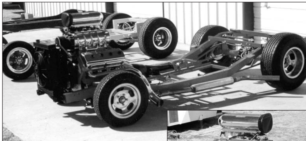
Top: Bob Carpenter's Henry J sits idle as it awaits the installation of its body. The engine, a 1957 or 1958 Chrysler Corp. Hemi, already has been mounted to the car's chassis. (Inset) Carpenter's reconstructed Henry J will have an engine similar to ones used briefly on the NASCAR circuit as well as some '50s era Chrysler vehicles. Photos courtesy of Carpenter
