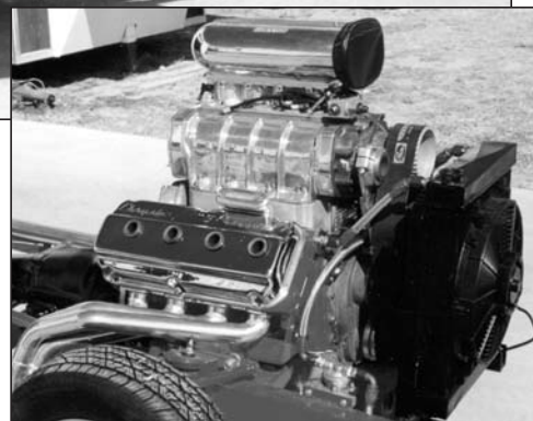
Top: Bob Carpenter's Henry J sits idle as it awaits the installation of its body. The engine, a 1957 or 1958 Chrysler Corp. Hemi, already has been mounted to the car's chassis. (Inset) Carpenter's reconstructed Henry J will have an engine similar to ones used briefly on the NASCAR circuit as well as some '50s era Chrysler vehicles. Photos courtesy of Carpenter
