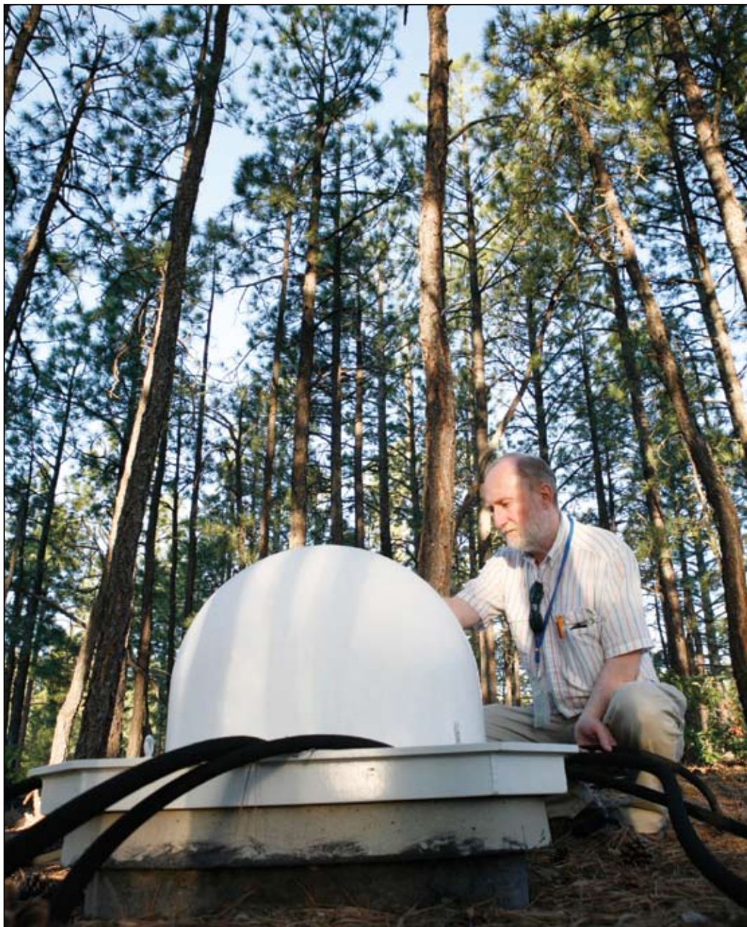
Laboratory researcher Doug ReVelle of Atmospheric, Climate, and Environmental Dynamics checks one of the infrasonic microphones in the woods near the Wellness Center in Technical Area 3 that were originally developed to listen for distant clandestine nuclear weapons tests. Over the past several decades, ReVelle and his collaborators have documented the explosions of hundreds of bolides in Earth's atmosphere, as well as other man-made explosions in the atmosphere. Photo by LeRoy N. Sanchez, Records Management/Media Services and Operations
