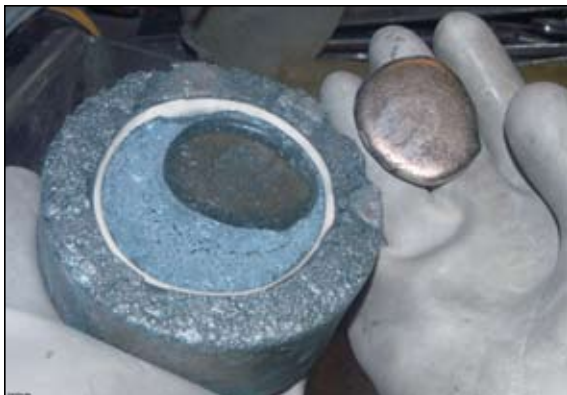
Impure plutonium metal (left photo in glove) is purified creating a 99.95 percent pure plutonium feed source (outer ring) which can then be alloyed (right photo) to produce the required chemical composition to make a pit. Photos courtesy of the Program Management (PM) Division
