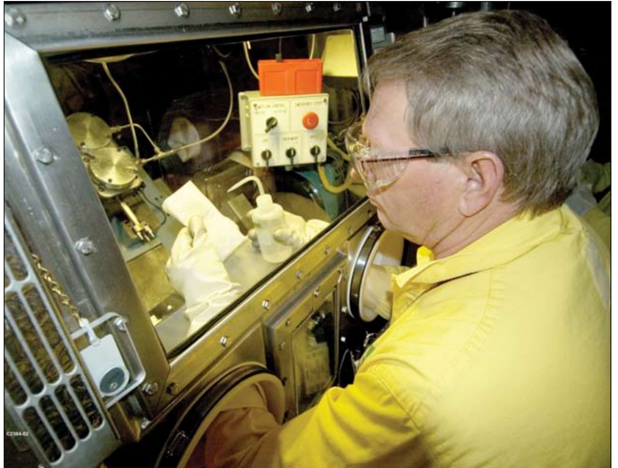
Literally taking thousands of hours to make, the use of Plutonium in Pit Manufacturing requires the specialized skills of a glovebox worker to cast, shape, inspect, and assemble the needed components into quality product.
