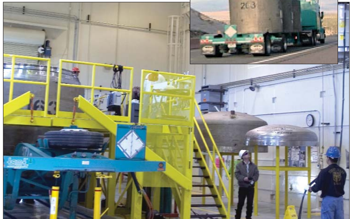
Workers at Los Alamos' Radioassay and Nondestructive Testing Facility load drums containing transuranic waste into a TRUPACT container. The TRUPACT is then bolted onto a flatbed. The first shipment in 18 months recently left for the Waste Isolation Pilot Plant. A TRUPACT container has a stainless steel skin over a 10-inch layer of polyurethane foam designed to absorb shock and resist fire. The containers are 10 feet tall and 8 feet in diameter. One TRUPACT can hold up to 14 waste drums, so a normal truckload of three containers can carry up to 42 waste drums. Inset photo, A truck carrying TRUPACT containers travels east on NM 502 with a shipment of waste headed for the Waste Isolation Pilot Plant in Carlsbad. Photos by Patricia Leyba, Environmental Stewardship (ENV) Division and John Bass, Public Affairs
