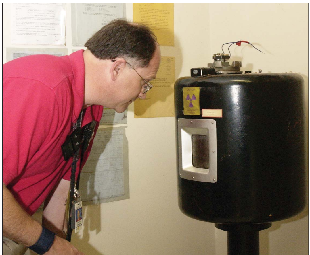
Andy Tompkins of Los Alamos' Offsite Source Recovery Project looks at a Gammator. The Gammators recently were removed from three Texas high schools, where they had been stored for more than 30 years after a brief career irradiating seeds, cells and other objects with gamma rays for school science experiments. Photo by LeRoy N. Sanchez
