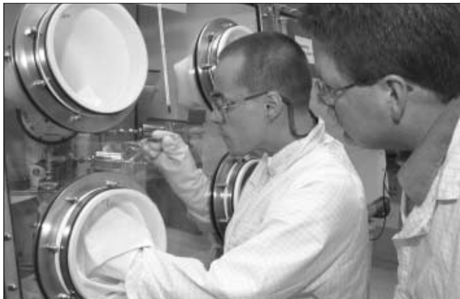
Anthony Lupinetti, left, of Actinide Processing Chemistry (NMT-2), and Kent Abney of Isotope and Nuclear Chemistry (C-INC) examine plutonium boride encased in a quartz tube at the alpha wing of Technical Area 48. Lupinetti's and Abney's work aims to produce a more stable form of plutonium suitable for longer-term storage.
