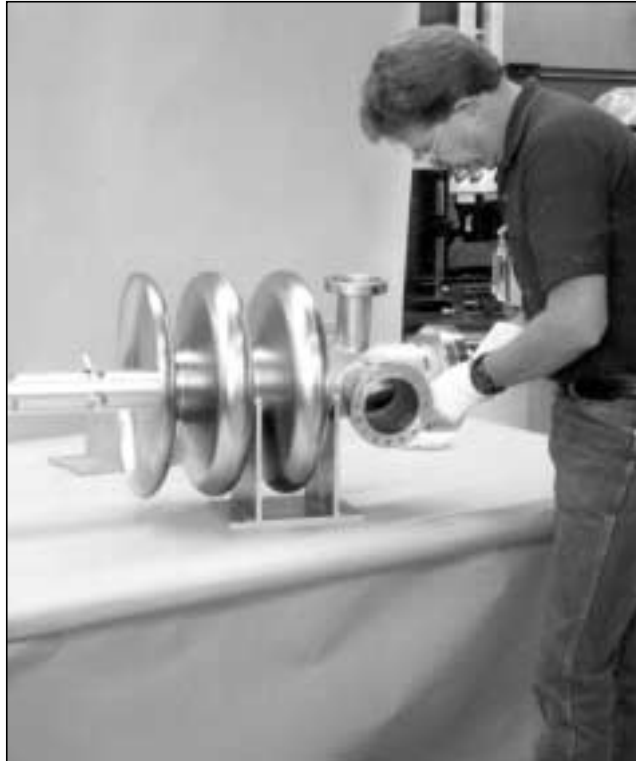
Frank Smith, a member of the welding team in Metallurgy (MST-6), inspects the weld he completed on the flange. In the next step, Smith prepares the piece for welding on the opposite side. The final weld is made in the center of the third cell, in the middle of the component. Smith performs 21 welds to complete one component. Photo courtesy of Mark Cola
