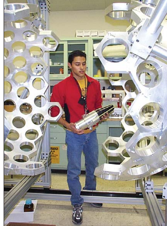
David Lujan of Neutron and Nuclear Science (LANSCE-3) displays a barium fluoride crystal, which is part of the Detector for Advanced Neutron Capture Experiment (DANCE). The experiment will be used to develop an understanding of the synthesis of chemical elements in stars, the burn-up of nuclear waste as well as an understanding of nuclear explosives from archived data. Lujan, an electro-mechanical student, is helping to get the project online. Photo by Michael Carlson
