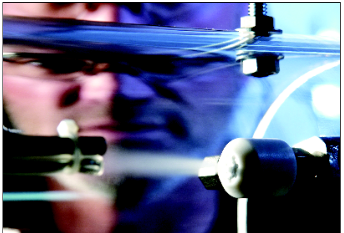
Jerry Barton of Applied Chemical Technologies (C-ACT) calibrates the temperature position of the carbon dioxide jet for Snow-Machining applications at a Technical Area 35 laboratory. The process could someday eliminate the use of oil-based or synthetic chemical fluids for metal cutting and metal parts cleaning in industry. Photo by LeRoy N. Sanchez
