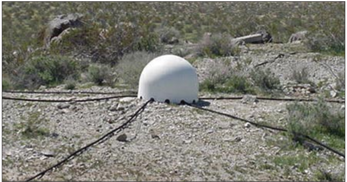
Detectors such as this infrasound array operated by the Laboratory have helped detect meteors and missiles and have played a key role in helping scientists determine the frequency by which giant meteors enter Earth's atmosphere. Photo courtesy of Atmospheric, Climate and Environmental Dynamics (EES-2)
