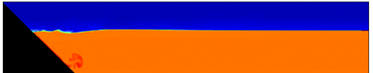
A two-dimensional tsunami calculation of a La Palma-type landslide event. Here the total wave amplitude is about 2 kilometers, however, the image also indicates a lot of wave-breaking and slide entrainment.
