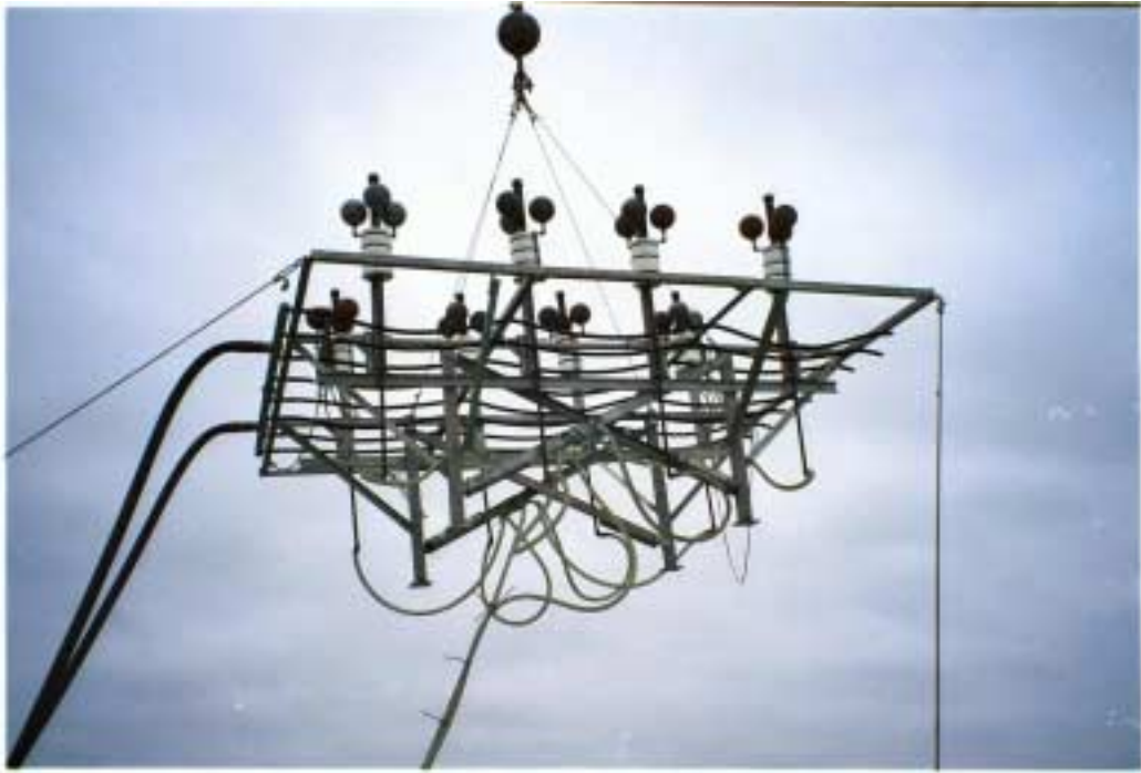
Figure 2 - New welded bubbler frame; note air nozzle telescoping mounts.
