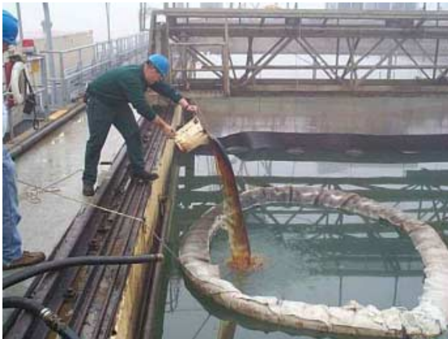
Figure 15 – SWEPI boom undergoing thick oil containment test.
