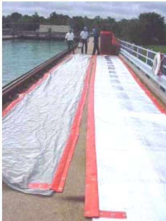
Figure 10 - Oil cooled fire blanket deck prior to its USS-42B boom
