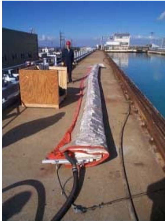
Figure 8 - Oil Stop, Inc. Auto Boom Fire Model on deck.
