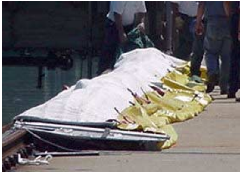
Figure 9 - Elastec/American Marine water-cooled fire blanket installed on the USS-42B boom.
