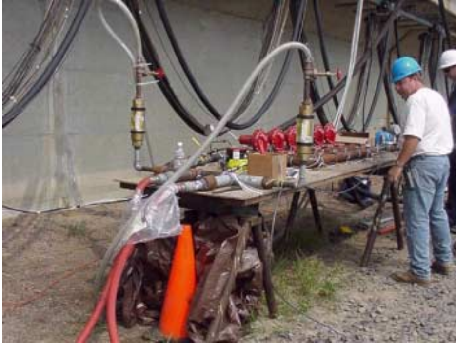
Figure 4 - propane regulator bank and compressed air manifold valves.
