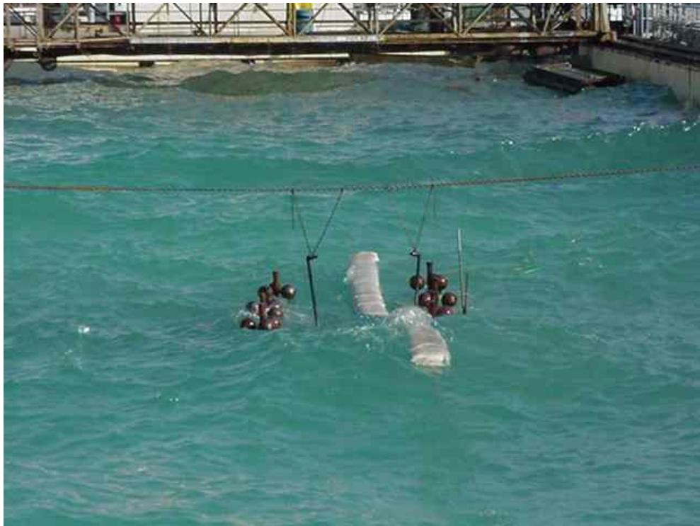
Figure 17 - Wave over-topping SWEPI boom.
