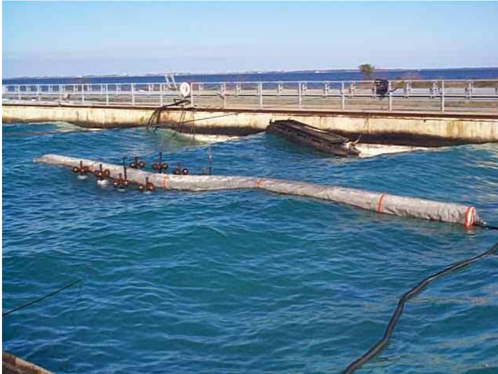
Figure 42 - Oil Stop Auto Boom during Pre-burn Wave Stress test.
