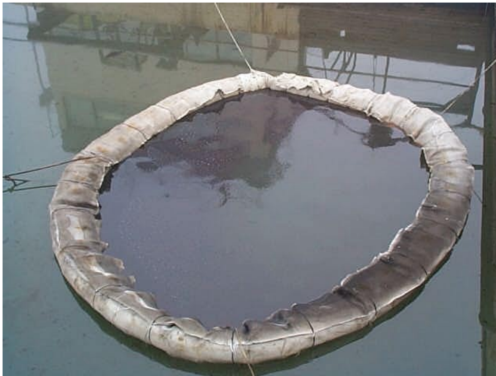
Figure 41 - SWEPI boom static oil containment test.
