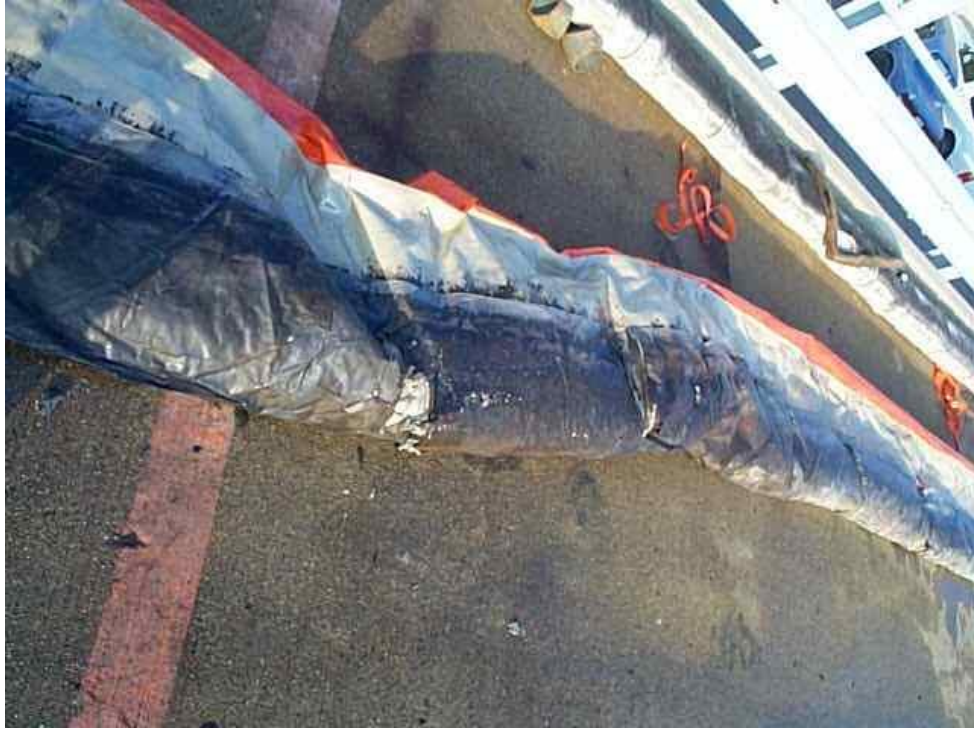
Figure 60 - Boom on deck showing exterior damage.
