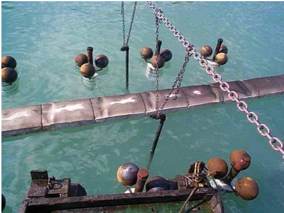
Figure 29 - Close-up of SWEPI boom after first cool-down.
