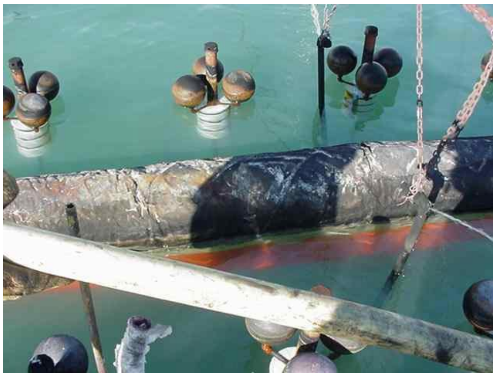
Figure 53 - Close-up of Oil Stop boom after first burn.
