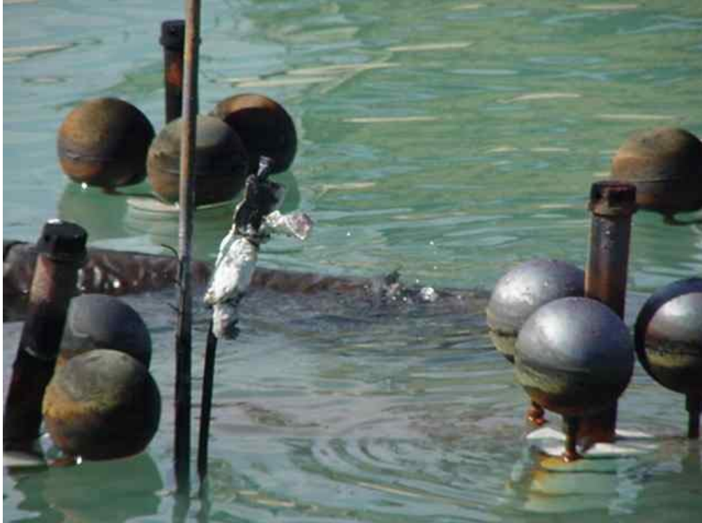
Figure 9 - Instrument stalk supporting ignitor and flame thermocouples
