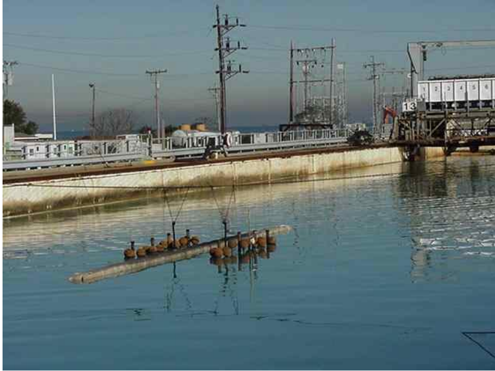
Figure 34 - SWEPI boom after second hour cool-down.
