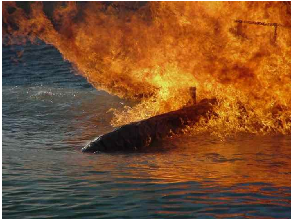
Figure 47 - Close-up of Oil Stop boom during first hour of flame exposure.
