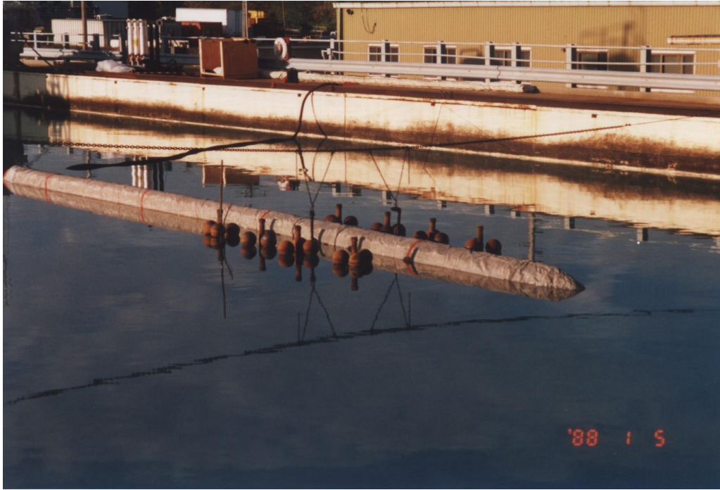
Figure 7 - Boom deployed in tank for pre-burn wave stress test.
