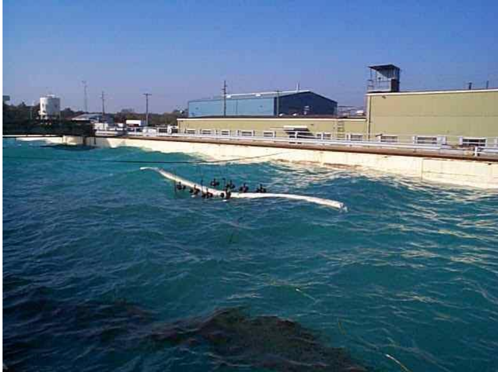
Figure 16 - SWEPI boom in waves.
