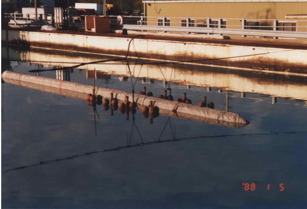
Figure 44 - Oil Stop Auto Boom after Pre-burn Wave Stress test.
