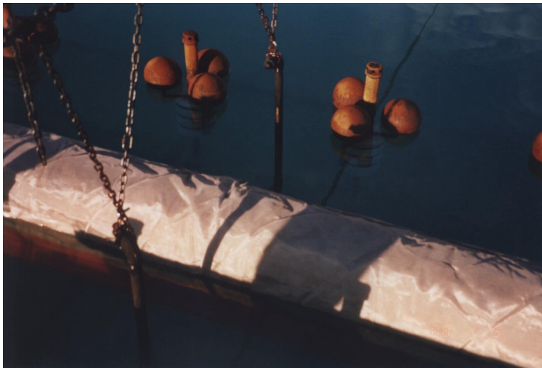
Figure 45 – Close-up of Oil Stop Auto Boom after Pre-burn Wave Stress test.
