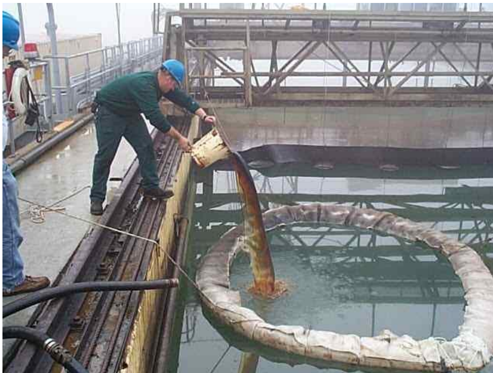
Figure 10 - Boom undergoing thick oil containment test.
