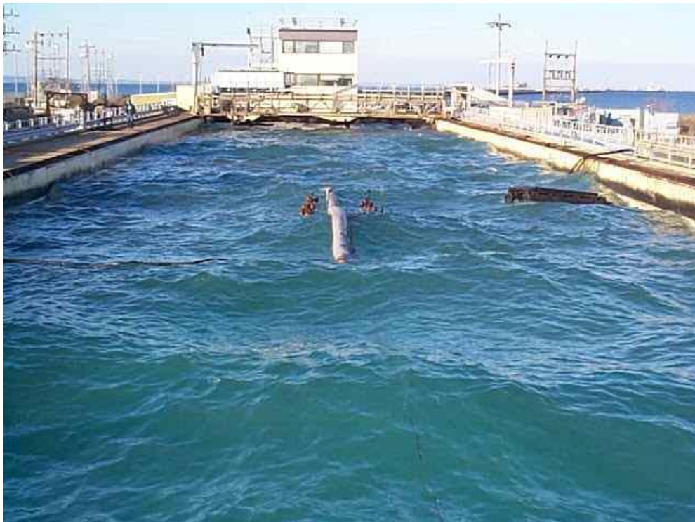
Figure 43 - Oil Stop Auto Boom during Pre-burn Wave Stress test.
