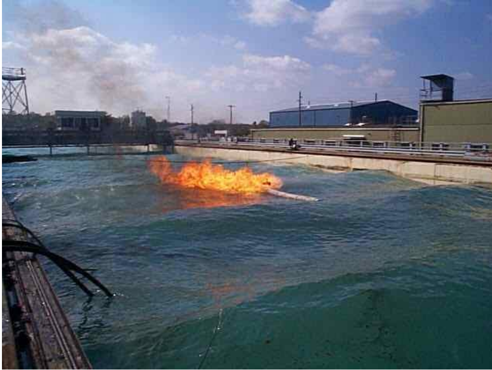
Figure 22 - Photo of SWEPI boom during first hour of flame exposure.
