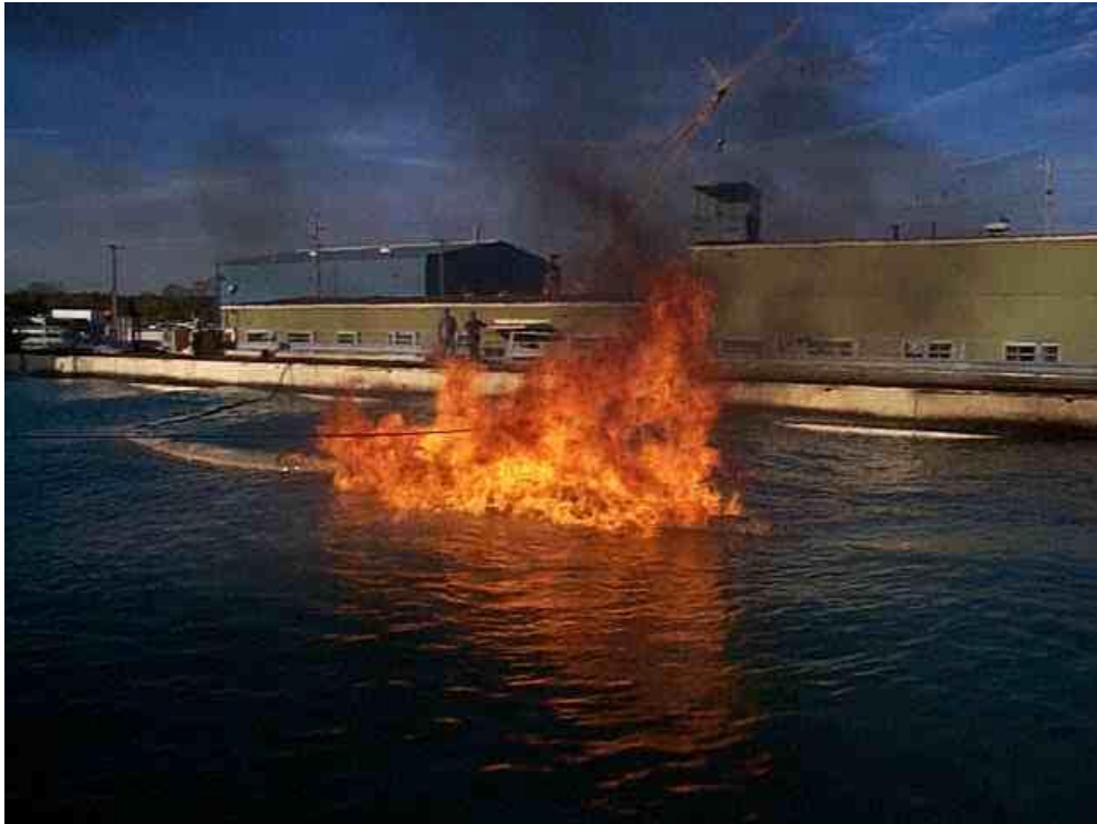
Figure 7 - Boom deployed in tank for pre-burn wave stress test.
