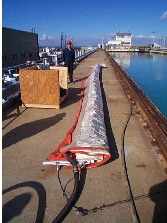
Figure 12 - Oil Stop, Inc. Auto Boom Fire Model on deck.
