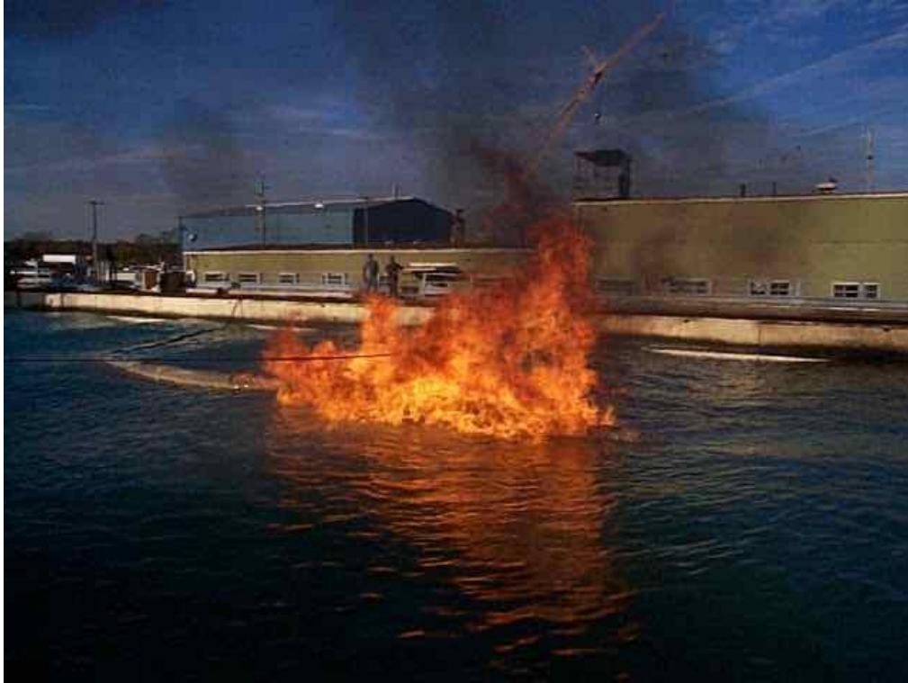
Figure 46 - Photo of Oil Stop boom during first hour of flame exposure.
