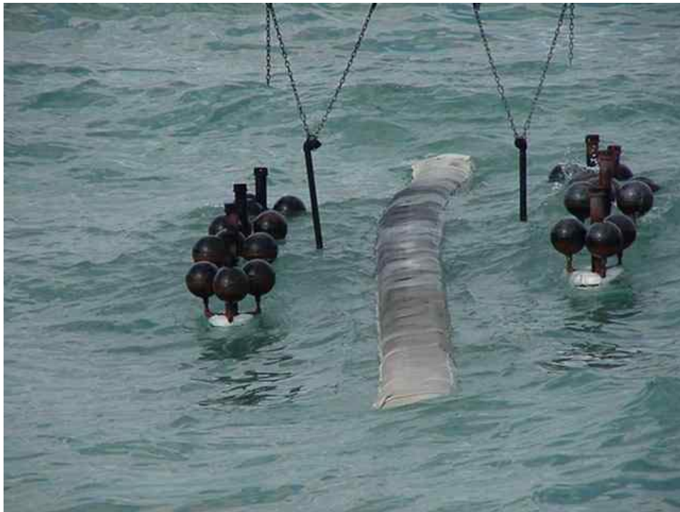
Figure 35 – Close-up of SWEPI boom during second hour cool-down.
