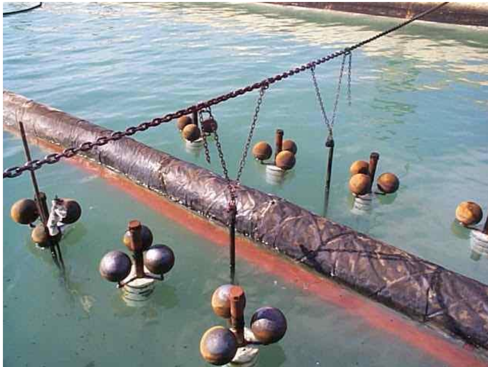
Figure 52 - Oil Stop boom after first burn.
