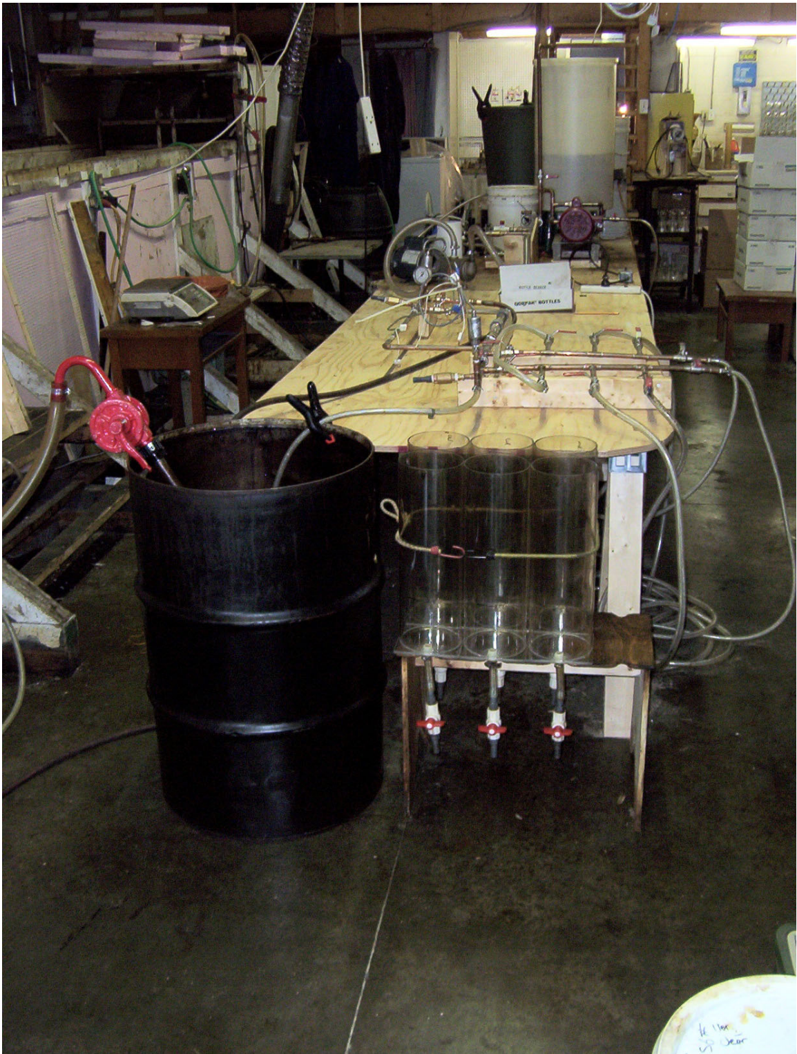
Figure 2-5. Photograph of laboratory scale-model piping system.
