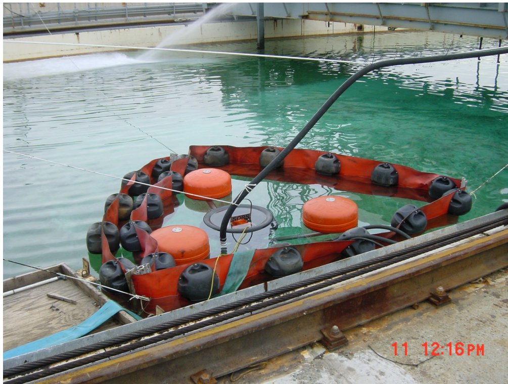
Figure 3-2. Photo of boom triangle and Desmi Terminator skimmer in water.
