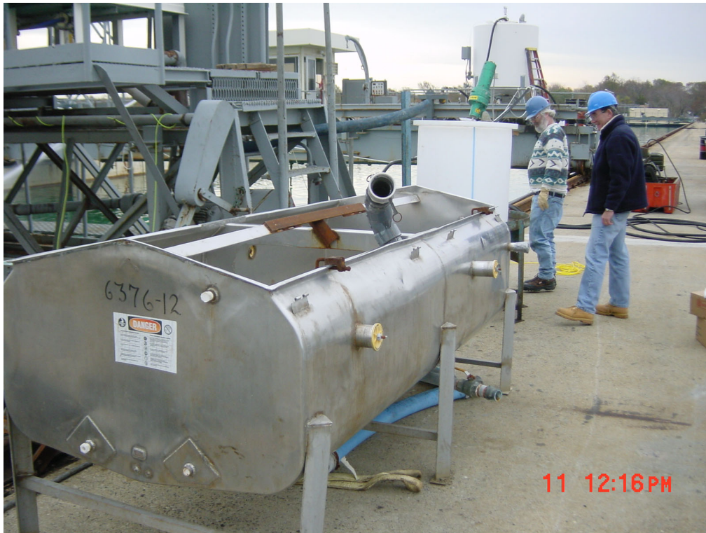
Figure 3-4. Decanted water temporary storage tank (foreground) and water sampling tank (background)
