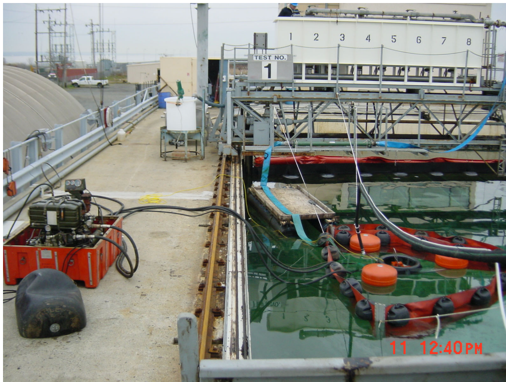
Figure 3-2. Photo of boom triangle and Desmi Terminator skimmer in water.
