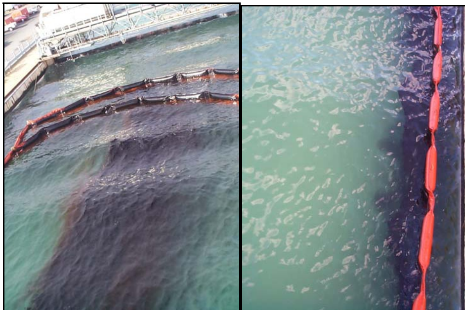
Figure 3-10: Photos of Dispersion in Tests #17 and #18
