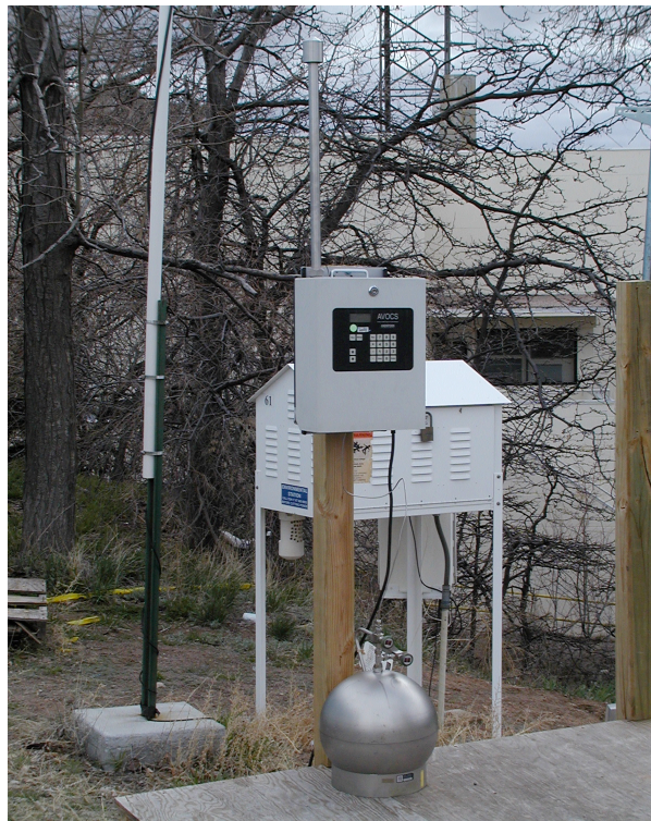
Figure 4-2. Ambient Volatile Organic Collection System at Site #61.
