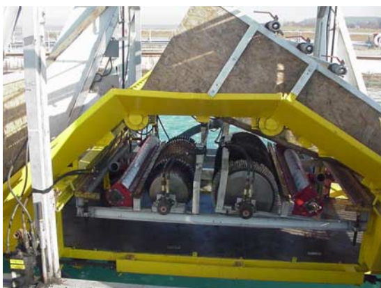
Brush-drum recovery unit installed, side-walls removed.
