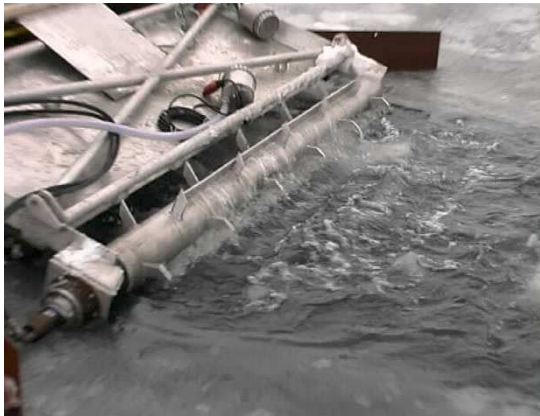
Ice feeder being operated in the pool after attaching paddles to the spikes.
