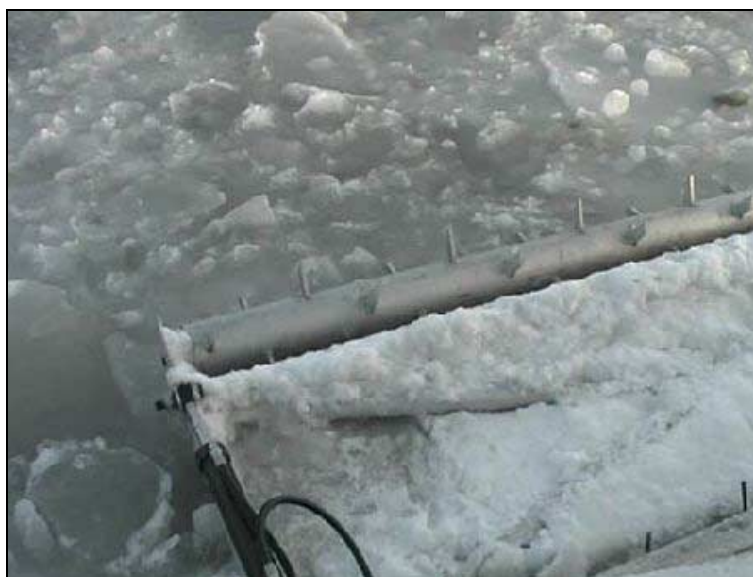
Figure 4.8 Ice feeder operating in broken ice. Snow covers the frame with the aluminum plate.
