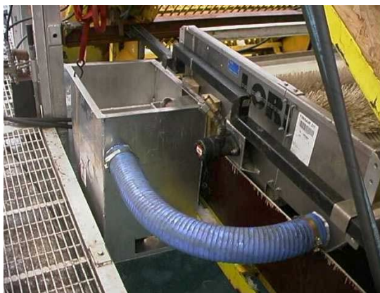
LORI unit seen from starboard side. The DOP 250 pump located inside the hopper.
