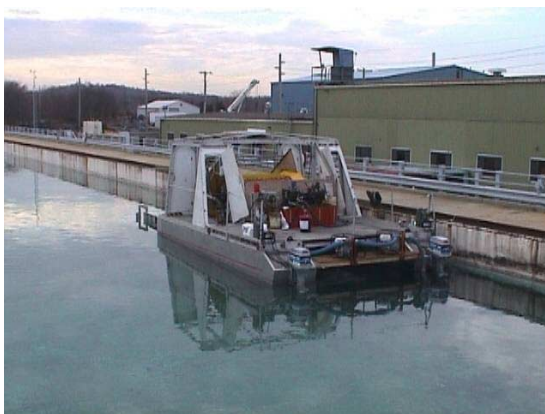
Work platform in the test tank. All equipment is not installed, hence the vessel has a forward trim.
