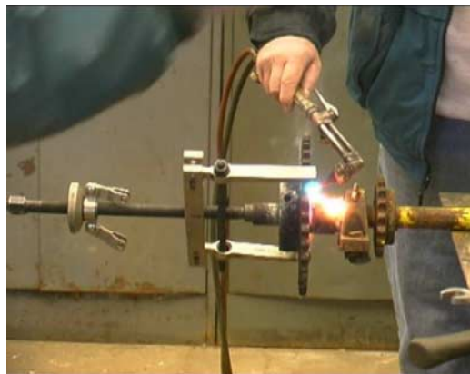
Driveshaft for the LGB removed. Heating was necessary to change the sprocket for the motor in order to increase the pulling force of the belt.
