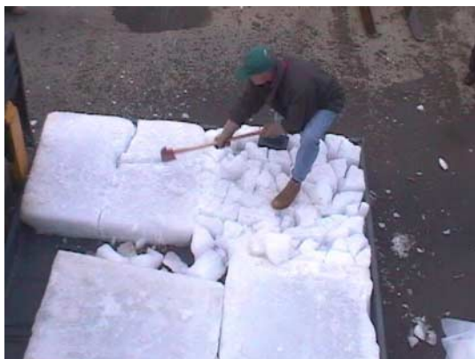
Ice being chopped in various sizes prior to deployment in the test tank.
