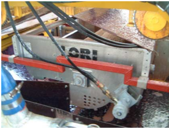
Plate on the side of the unit guides oil and ice to the inlet of the recovery unit. Another plate on the top prevents ice from falling into the rear trough.
