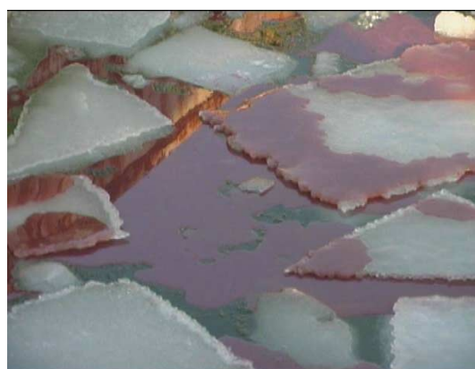
The oil is dyed red to be more visible.
