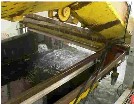
The flushing system being operated after increasing the cross section of the flow-lines. Water enters the recovery area from both sides of the trough.
