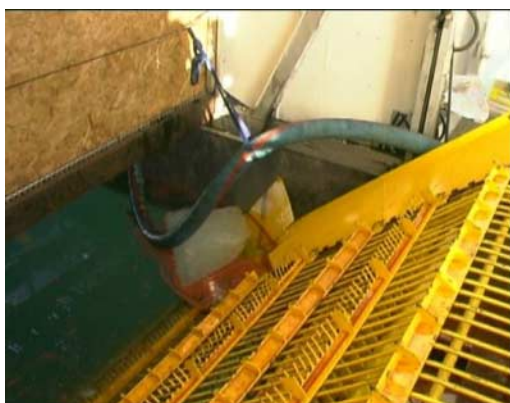
A hinged plate at the rear closes the opening between the hull and the LGB.
