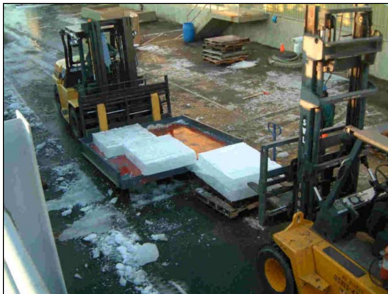
Figure 4.2 Placing ice slabs on the steel platform for deployment.
