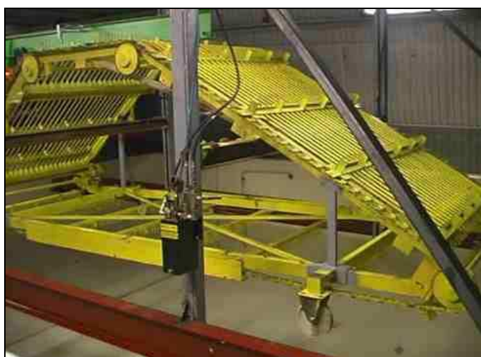
Figure 4.10 A stripped version of the Lifting Grated Belt installed in the HSVA test tank.
