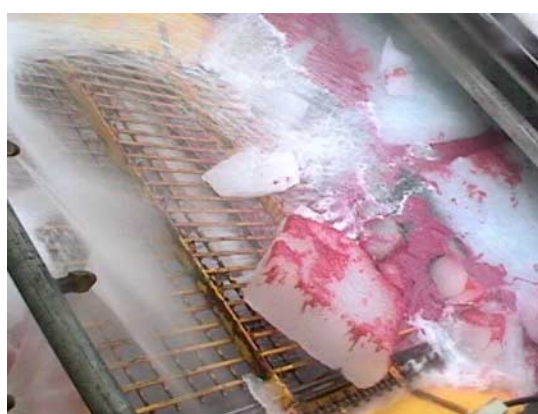
Contaminated ice being deflected over the belt where water from the spray nozzles will flush off the oil.
