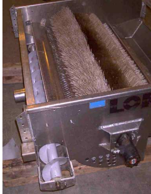
Figure 4.13 Auger installed in the rear trough of the LORI unit.
