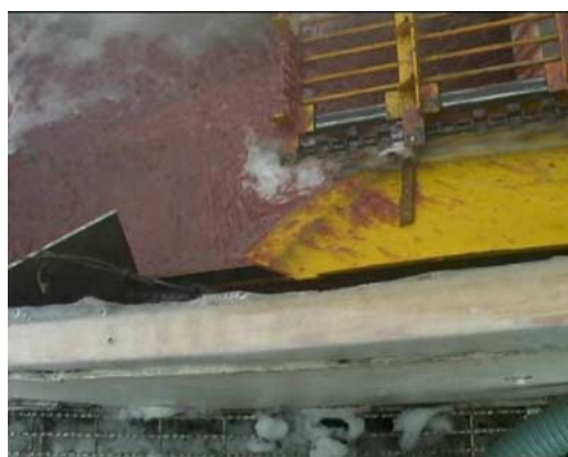
Flushing water sliding down the side plate of the LGB is pushing oil away from the belt. A piece of wood reduces the negative effect to some extent.
