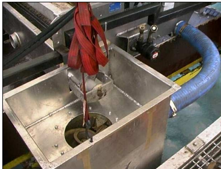
Figure 4.14 DOP 250 pump installed in hopper connected to auger and front trough.
