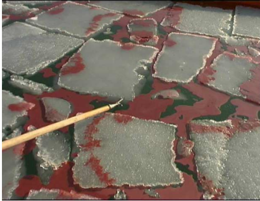
Oil distributed in the ice field. There has been some ice formation overnight, see the rim of the ice pieces. Frazil ice between larger ice.
