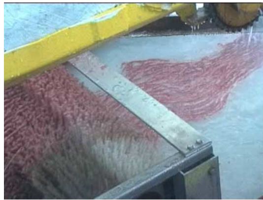
Due to lots of turbulent flushing water entering the recovery area, the oil is forced to the central part of the cylindrical brush.
