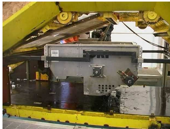
The LORI recovery unit installed in the LGB, side-walls not in place, port side.
