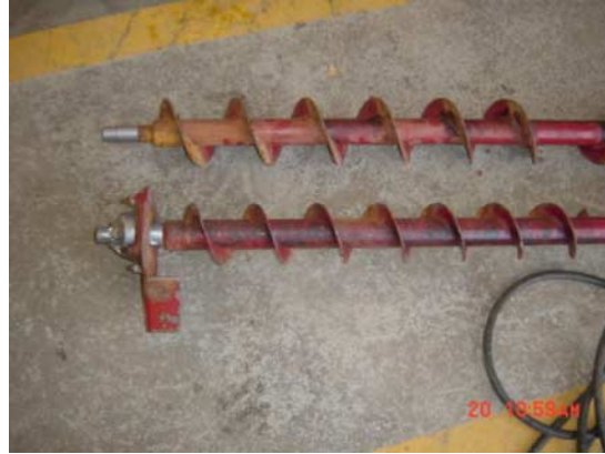
Most of the steel parts were heavily corroded, here the augers are disassembled for painting.
