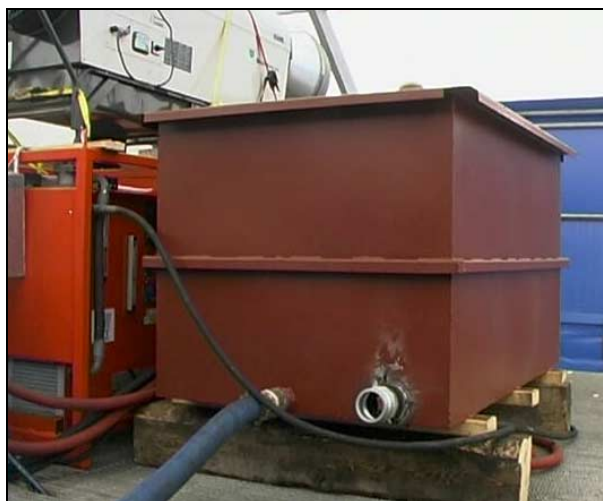
Figure 3.2 Tank for recovered product, 1300 l.
