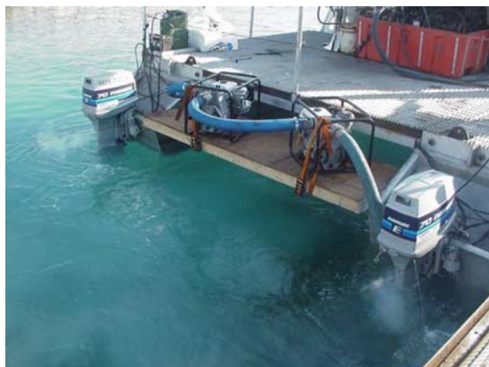
Pumps for water flushing installed in series on the rear platform. The hose from the pumps to the spraybars runs under the main deck.
