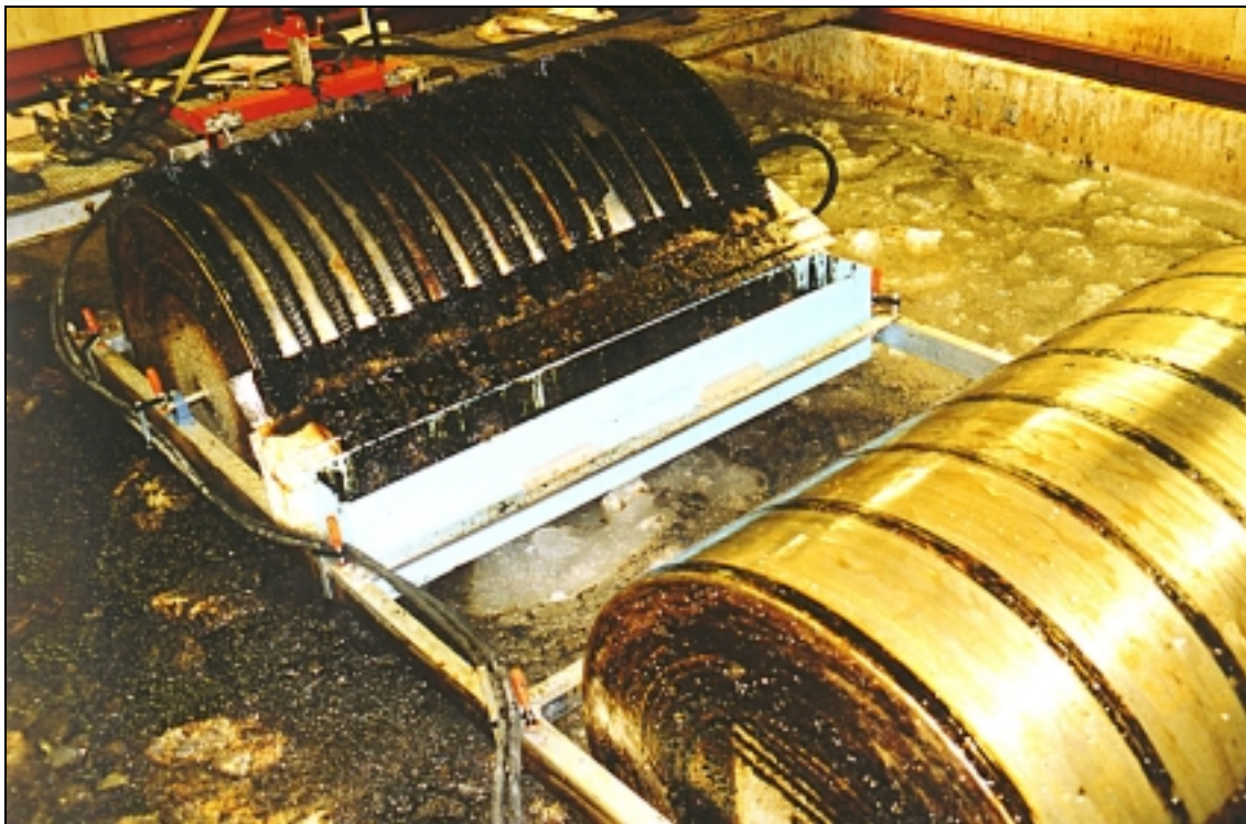
Stainless steel brush/drums in wet test with oil and ice.
