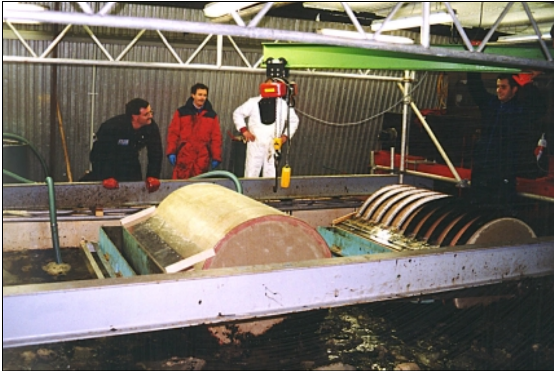
Large brush drum system installed in the test tank, Configuration 1 with two large drums. Smooth drum to the left, brush drum with two different materials to the right, both drums of composite material.
