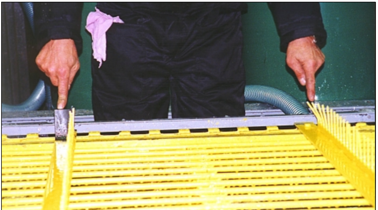
Reinforced rake tine (left), rake tines before reinforcement (right).
