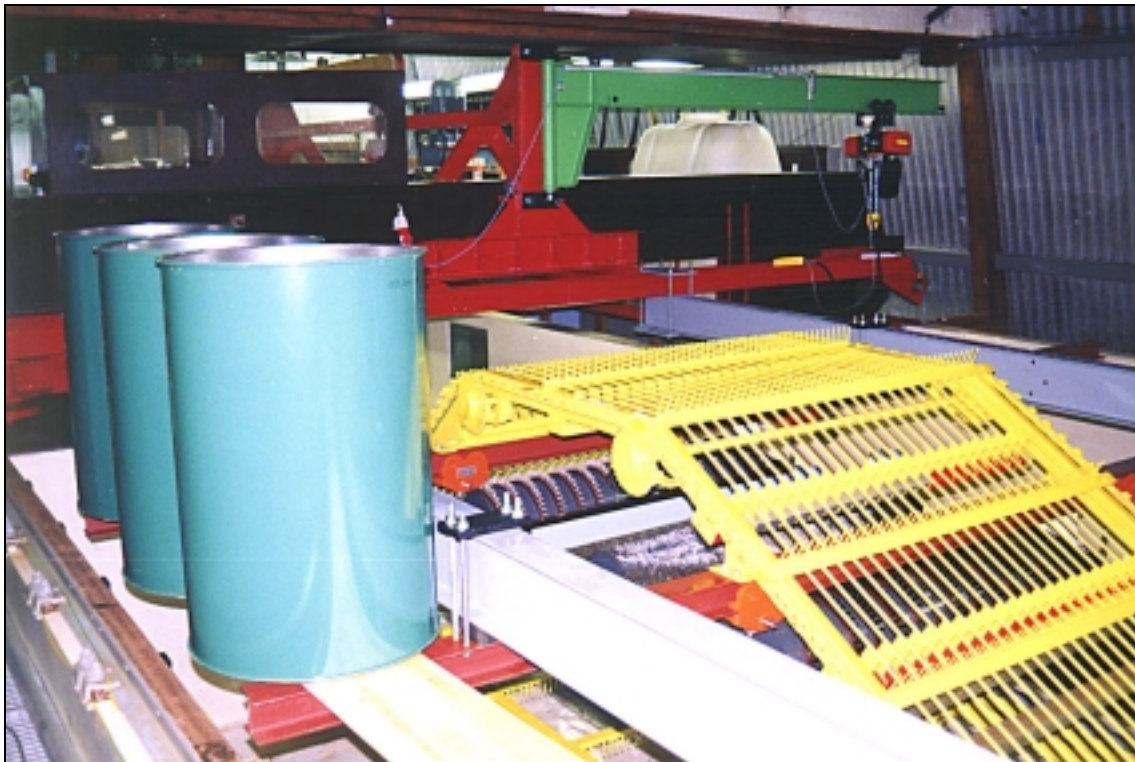
LGB installed in the test tank, supported by I-beams. Small brush drums underneath the belt, green barrels for recovered product to the left. In the background the main carriage with crane (green beam with winch) and flushing water tank (white).
