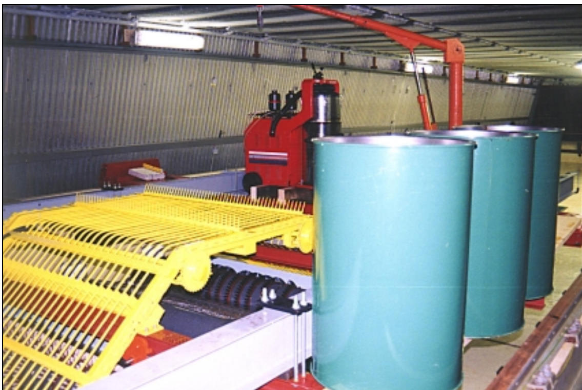
LGB seen from the other side. Secondary carriage with crane and air conveyor in the background.
