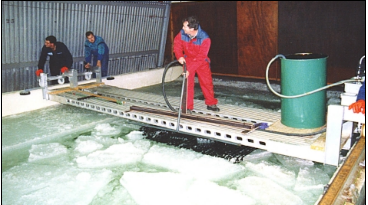
Initial method to distribute the oil in the tank.
