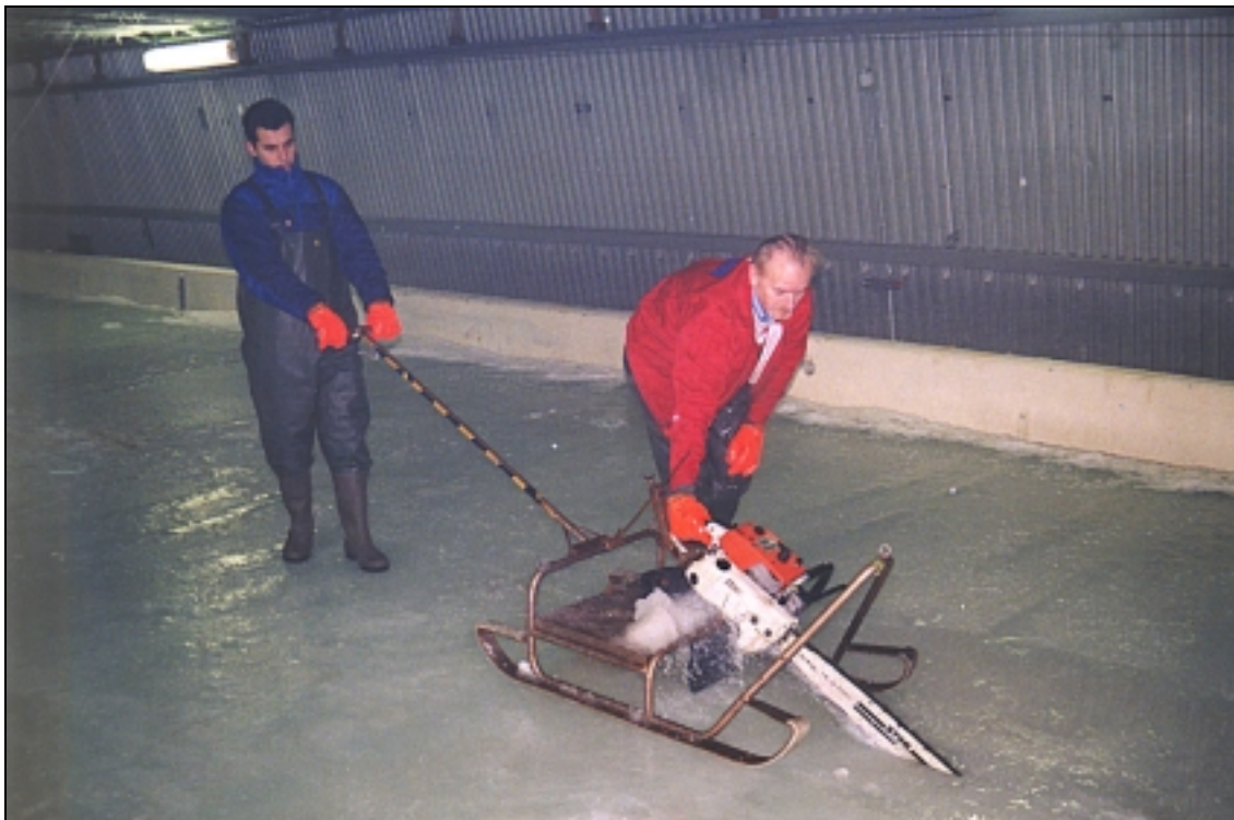
Cutting the ice in the HSVA test tank with a chain saw before starting the testing.
